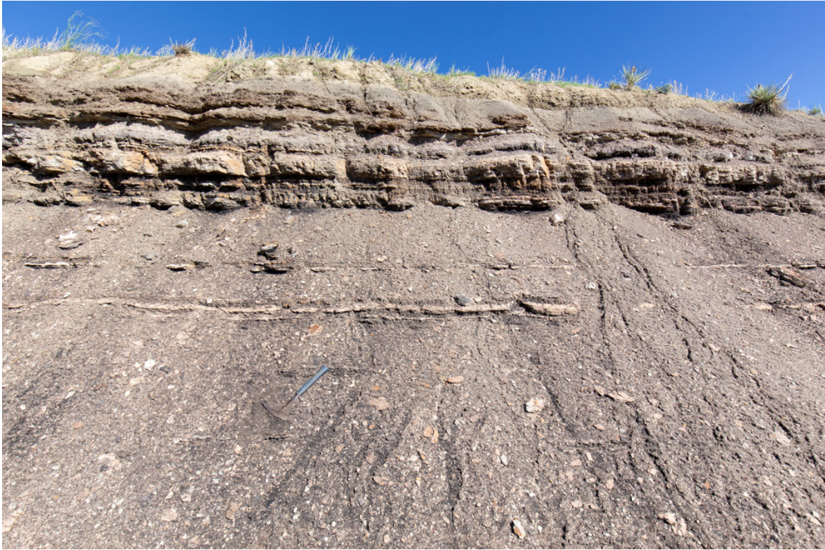
Photo of the eroded Denver Formation lignite roadcut prior to sampling. Interbedded sandstone, claystone, carbonaceous shale, and smaller lignite beds cap the slope-forming lignite. More resistant and relatively thin (2- to 3-inch thick) tonstein/clay layers form continuous ledges on the slope (e.g. center of photo, above the hammer) within the eroded lignite.
