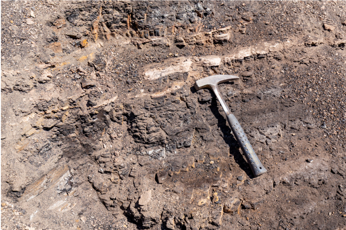
Figure 9 – Close-up photo of the clay and/or tonstein layers shown in Figure 6 (hammer is ~13-inches long).
