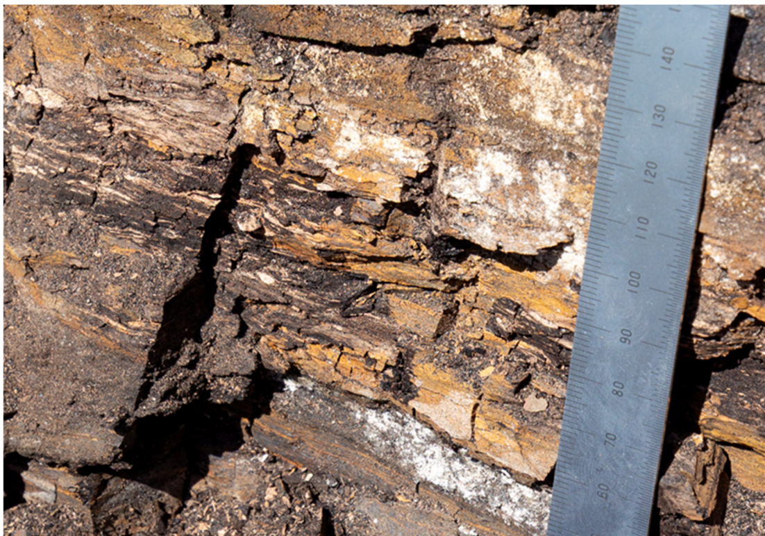
Figure 7 – Close-up photo of the Denver Formation lignite exposure (scale is in millimeters) showing fractured nature of the lignite, iron oxides, and gypsum (white).
