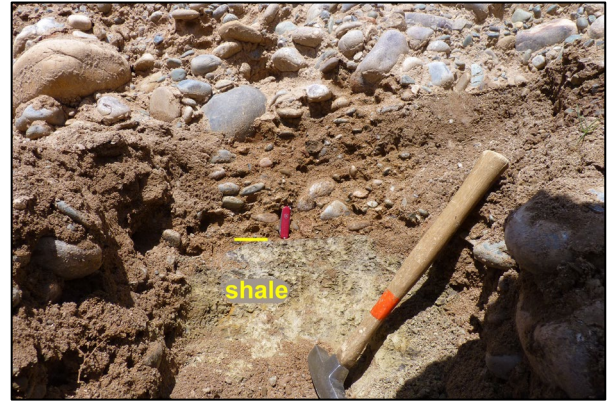
Figure 14—Basal contact (red knife) of fluvial gravel on shale bedrock in Hocker pit; lowest bed is pebbly sand overlain by cobble-pebble gravel.
