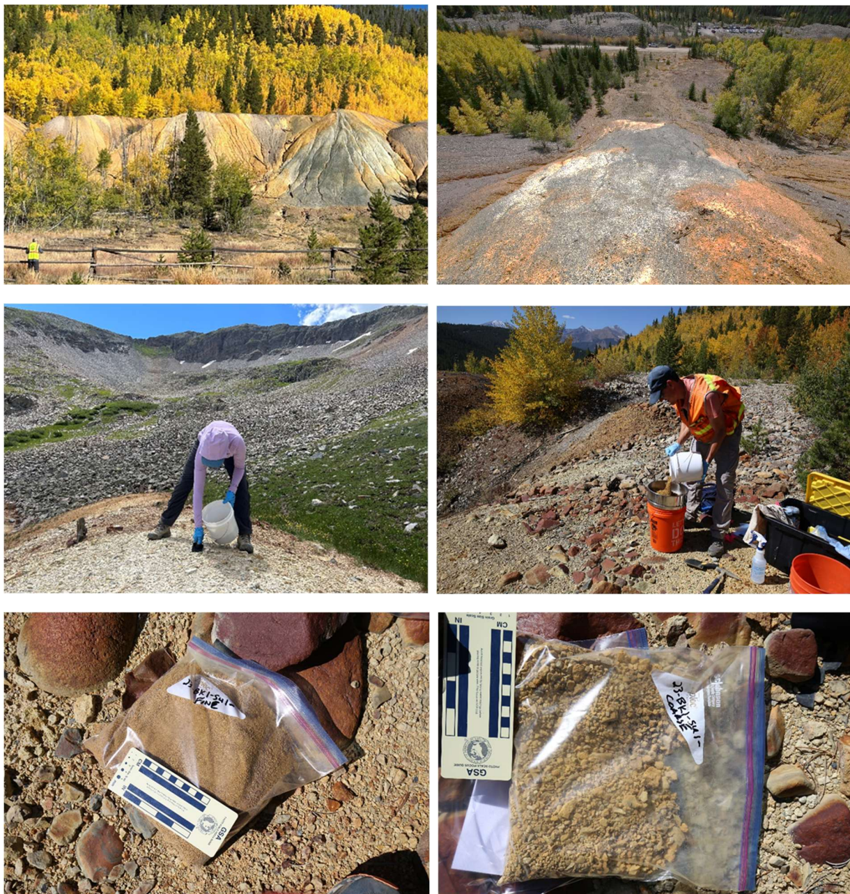
Figure 2 – Photographs showing the mine waste sampling procedure. Upper left and right – mine waste pile at Breckenridge, CO (Wellington Mine, Extenuate Adit). Middle left and right – mine waste pile grid sampling, compositing, and sieving (2 mm stainless steel sieve). Bottom left and right – fine (<2 mm) and coarse (> 2mm) composite samples.
