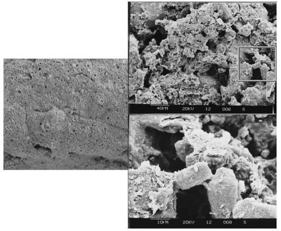
Figure 3. Hand sample on left at normal scale shows visible macro-pores in soil. SEM scan of clayey silt (CL-ML) on right shows abundant micro-pores and high void-space ratio. Close-up scan (scale bar in microns) on bottom right was taken from boxed area above. Note clay bridges supporting silt grains. SEM images courtesy of R. Luehring.
