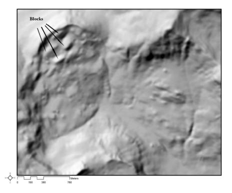
Figure 3. Portion of the 10 m DEM of the head of West Lost Trail Creek valley, about 2.9 km upstream of the 1991 West Lost Trail Creek landslide. Note that blocks greater than 100 m wide are easily discerned (arrows).
