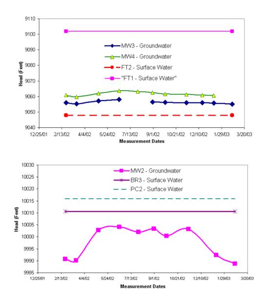
Figure 6. Hydraulic head for ground water and surface water at (top) Frisco Terrace, (bottom) Blue River Estates. Elevation reference is mean sea level. Average head at MW-1 is 10291 ft (not shown).
