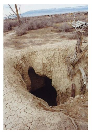
Figure 2. Sinkhole in clay alluvial soil as a result of soil dispersion and piping near Montrose, Colorado.
