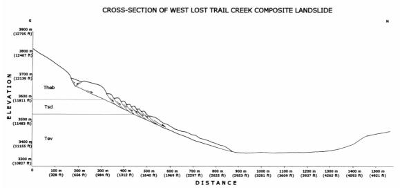
Figure 8. The 1991 West Lost Trail Creek landslide appears to have initiated as a series of retrogressive rotational rock slumps, progressing upslope over a 10 to 15-minute period (Rogers et al., 1999). The material below el. 11, 975 ft (3650 m) had previously been involved in land slippage.
