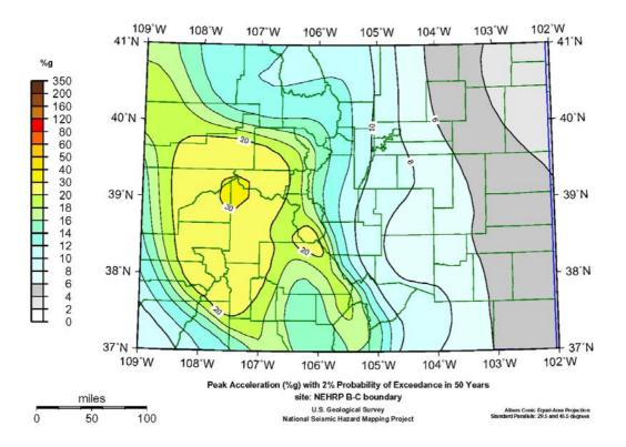
Figure 2. Expected earthquake accelerations with 2% Probability of Exceedance in 50 years (from USGS, 2003).
