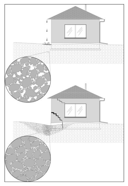
Figure 1. Schematic drawing of mechanical hydrocompaction. Soil skeletal fabric has lost volume from wetting and re-orienting of soil grains, which results in settlement at the surface. From White and Greenman (in prep.), used by permission.
