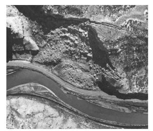
1967: Photo shows old Highway 6 and 24 passing through toe of landslide.
