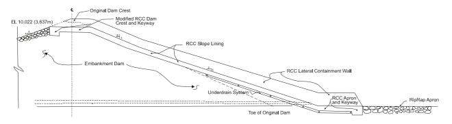
Figure 2. Modifications to downstream slope of the dam. Maximum cross section.
