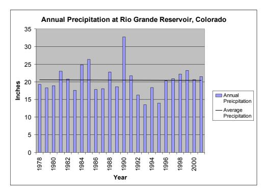
Figure 7. Annual Precipitation at the lower end of Rio Grande Reservoir (at the Farmers' Union Dam), about 10 miles downstream of the 1991 landslide. Note the extra normal rainfall that occurred in 1990, the year preceding the landslide.
