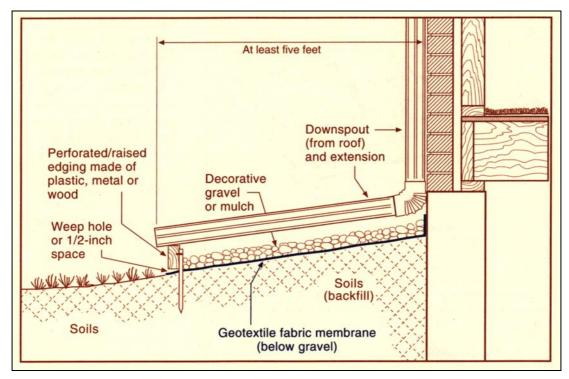
Figure 22. Landscaped runoff slope next to a house foundation. The roof drainage is carried by a downspout extension to a point beyond the slope. From Noe and others (1997); modified from Holtz and Hart (1978).
