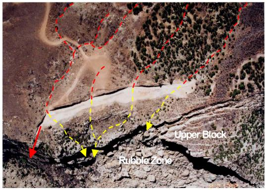
Figure 22. Water diversion structure constructed in Summer and Fall of 2003 to intercept drainage basins above landslide. Dashed red line of existing channel locations become dashed yellow where intercepted. Red arrow shows out-fall of diversion ditch over canyon rim to unnamed box canyon east of the landslide complex. Note that original drainage channels flowed into the Rubble Zone. Aerial photo courtesy of Robert Florez and the CDOT aerial reconnaissance unit.
