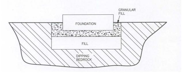
Figure 5. Typical subexcavation for footings in dipping bedrock.
