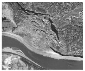
1958: Photo taken shortly after 1958 re-activation of landslide. Photo shows re-alignment of Highway 6 and 24 and grading of landslide slope.
