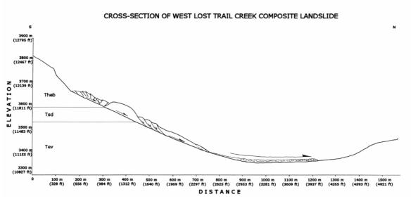
Figure 10. The rock flow emanating from the lower slope soon detached itself and speed across the valley floor as a sturzstrom, moving about 35 m/sec (Rogers, et al., 1999). A much greater portion of the landslide translated 100 to 300 m, but remained on the slope.
