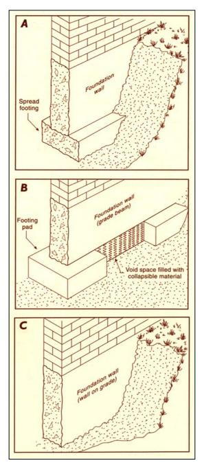
Figure 14. Shallow footing-and-wall type foundation systems. (A) Spread footing. (B) Discontinuous footing pad. (C) Wall-on-grade. From Noe and others (1997); modified from Holtz and Hart (1978).
