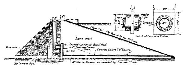
Figure 8. Castlewood Dam; cross section through intake/outlet works and upstream berm after reconstruction (Schuyler, 1909).
