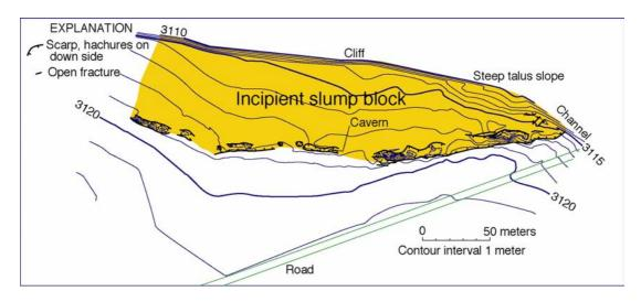
Figure 5. Fractures and other surface features of an incipient slide block near Crater View.
