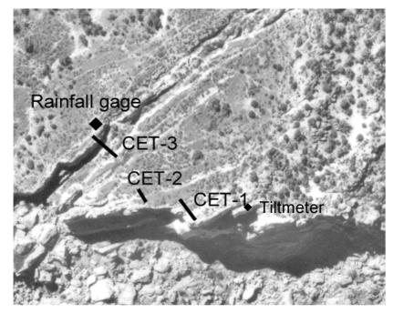
Figure 9. Close-up aerial photo of main graben and Upper Block with locations of cable extensometers (CET), tiltmeter, and base station that includes a rainfall gage.
