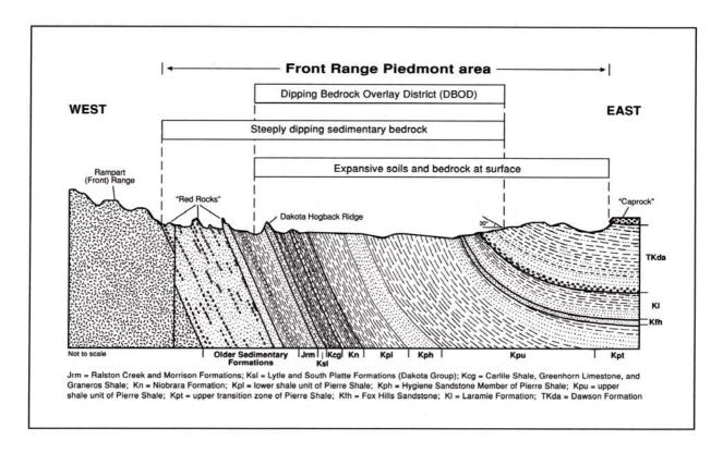
Figure 2. Schematic cross-section of geologic formations in northwestern Douglas County, showing expansive and steeply dipping bedrock zones. From Noe and Dodson (1999).
