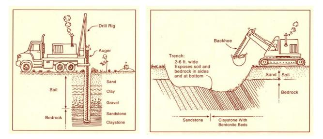
Figure 4. Methods for assessing subsurface geology: (A) Drilling. (B) Trenching. Modified from Noe et al. (1997).
