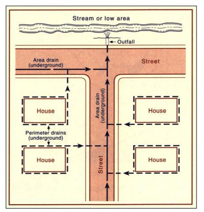
Figure 20. Map view of a typical area drain layout. From Noe and others (1997).
