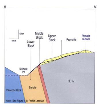
Figure 9. Pre-displacement geotechnical model profile.
