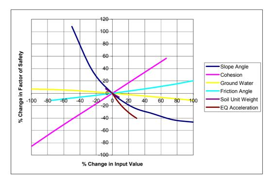
Figure 9. Sensitivity analysis of variables influencing stability for small slopes (< 100 cubic yds or 75 cubic m). Input variables were modified and the effect on factor of safety against sliding was monitored.
