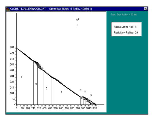
Figure 1. CRSP slope profile window (with rockfall simulation in-progress).
