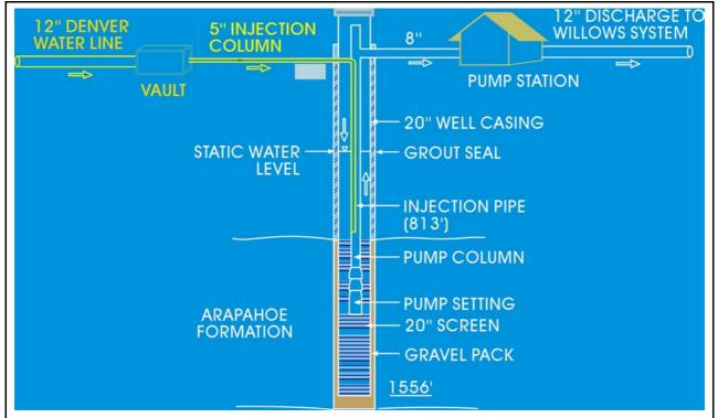
Figure 3. Production Well Completion and Injection Retrofit
