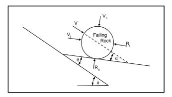
Figure 2. Impact angle ( $\alpha$ ) defined as a function of rock trajectory, slope angle ( $\phi$ ), and slope variation ( $\theta$ ). Rock velocity (V) is reduced into normal (V<sub>n</sub>) and tangential (V<sub>t</sub>) components. The tangential coefficient of frictional resistance (R<sub>t</sub>) and the normal coefficient of restitution (R<sub>n</sub>) act to decrease the falling rock's velocity (Pfeiffer, 1989; Pfeiffer et al., 1991; 1995).
