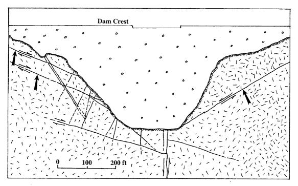
Figure 8. Gravity-slip surfaces (solid arrows) in granitic foundation rocks at Gross Dam, Colorado Front Range (after Wahlstrom, 1974). Faults of tectonic origin were present in the granite before the gravity-slip "faults" developed, and are geologically much older.
