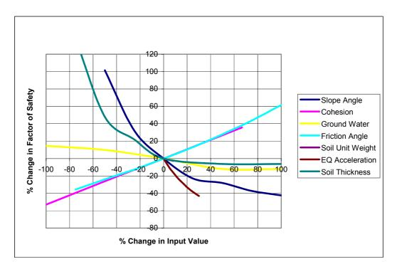
Figure 10. Sensitivity analysis of variables influencing stability for large slopes (> 10,000 cubic yds or 7500 cubic m). Input variables were modified and the effect on factor of safety against sliding was monitored.
