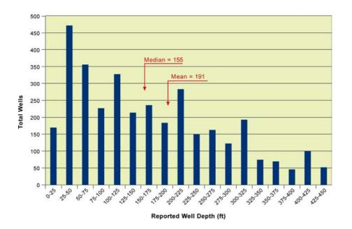
Figure 10. Histogram of well completion depths for the 90th percentile of wells completed in the Tertiary igneous rocks.
