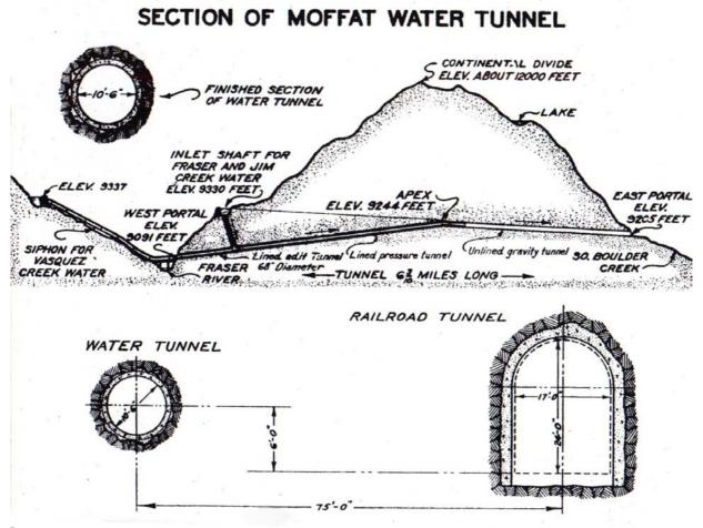
Figure 10. Profile and Section of the Moffat Tunnel.
