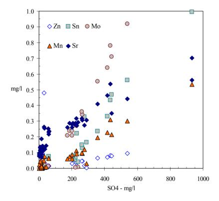
Figure 13. Plot of sulfate  $(SO_4)$  and trace metals in ground water and surface water samples. The data show increasing trace metal concentrations with increasing SO<sub>4</sub>, which likely reflect weathering of sulfide ore rocks.
