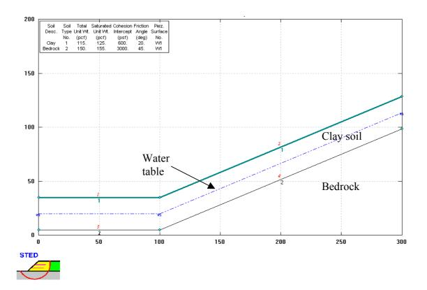
Figure 8. Typical slope profile analyzed for slope stability. The scale shown is for analysis of large slopes (200 ft or 60m long). Small slopes were also analyzed at 1/10 the scale shown.
