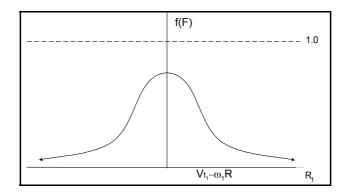
Figure 4. Friction function  $f(R_t, V_{t1} - \omega_1 R)$  as a function of the difference between tangential and rotational velocities (Pfeiffer, 1989; Pfeiffer et al., 1991; 1995).
