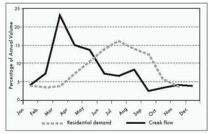
Figure 4. Plots of normalized stream-flow in Cherry Creek and residential demand show the outof-phase timing of surface water supply with demand (Colorado Geological Survey, 2002b - data courtesy Parker Water and Sanitation District).
