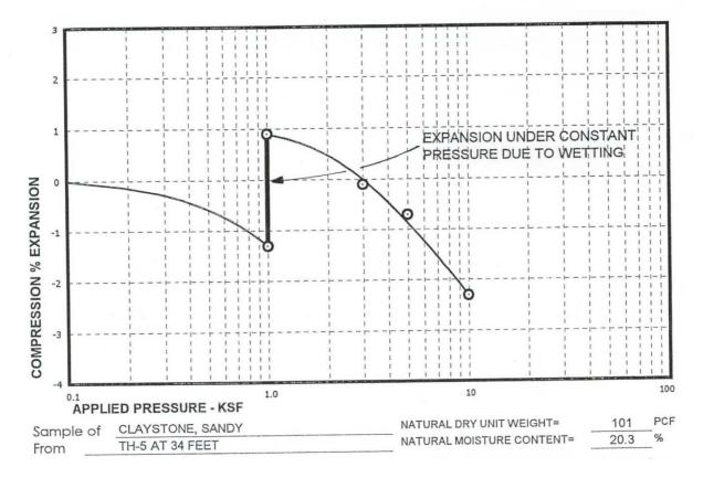
Figure 4. Typical swell-consolidation test plot.
