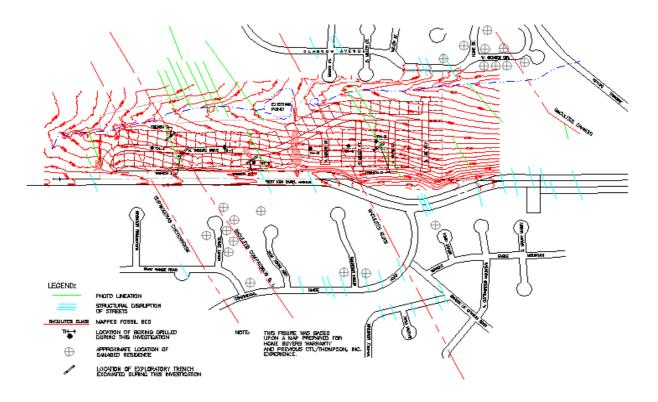
Figure 3. Evidence of geologic hazard in developed areas to the north and south of the Sanctuary, including damaged houses and linear heave features in streets (from CTL/Thompson, 1996).
