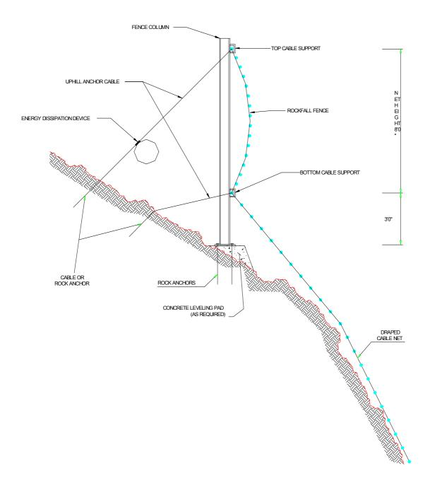
Figure 11. Profile of typical rockfall mitigation fence with draped cable net.
