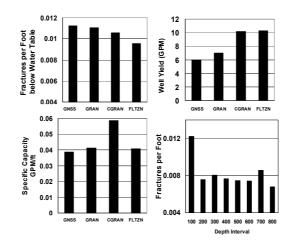
Figure 2. Hydraulic character of geologic units in Turkey Creek Basin: a) fracture frequency by rock group; b) well yield by rock group; b) specific capacity by rock group; and d) fracture frequency by depth interval (metamorphic gniess and schist, GNSS; granite, GRAN; coarse granite, CGRAN; and fault zones, FLTZN).
