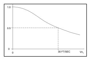
Figure 5. Normal coefficient scaling factor,  $B = \frac{1}{1 + \left(\frac{V_{n_1}}{30}\right)^2}$ , as a function of the incoming normal
