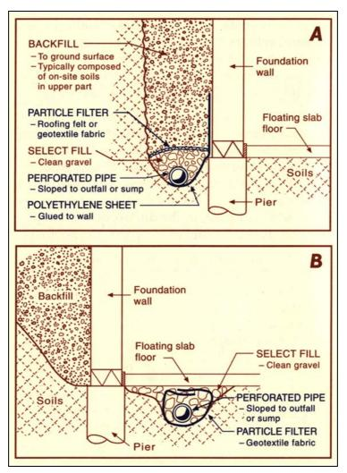
Figure 19. Components of a typical perimeter drain. (A) Exterior. (B) Interior. From Noe and others (1997).
