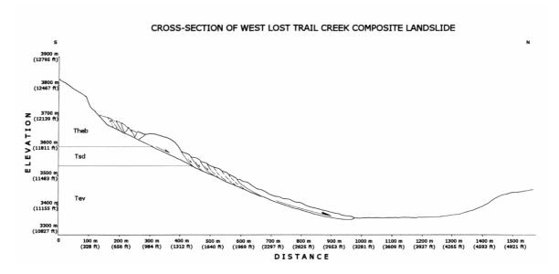
Figure 9. After the slumps joined together in a series of en-echelon blocks, the entire mass mobilized downslope, with an enormous rock flow progressively detaching from the upper mass and moving downslope onto the valley floor.
