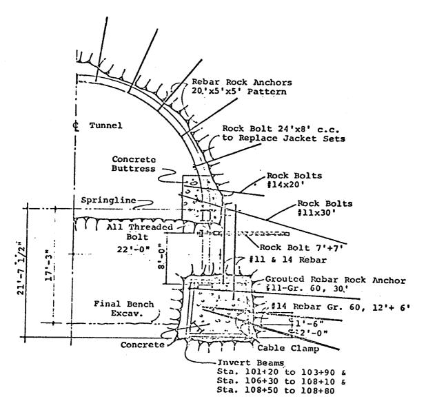
Figure 5. Zone III Rock Reinforcement and Support Sta. 100+30 to Sta. 109+07.
