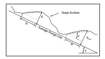
Figure 3. Surface roughness (S) established as the perpendicular variation from an average plunge line (defined by slope angle  $\phi$ ) over a distance equal to the radius of the rock (R). Maximum slope variation ( $\theta_{max}$ ) is defined by S and R (Pfeiffer, 1989; Pfeiffer et al., 1991; 1995).
