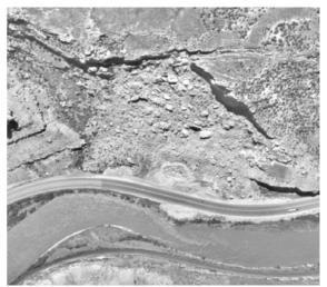
1999: Photo shows repair and buttressing of Interstate 70 following the 1998 re-activation of the landslide. Note darker asphalt where road repair occurred.
