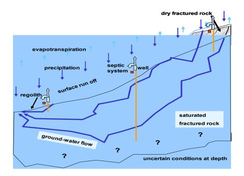
Figure 8. Envisioning the hydrologic cycle for a contained, fractured-rock basin facilitates understanding of the dynamics that need to be considered in water budgets.
