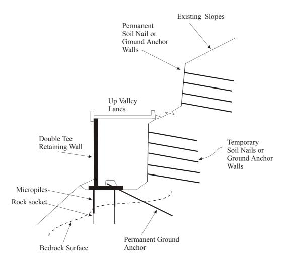
Figure 12. Generalized Profile of Retaining Wall with Micropile Foundation.
