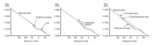
Figure 4. Schematic of raveling failure at cut slope in Type 3 and 4 rock.
