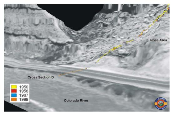
Figure 16. Cross Section D at east rotational area. Model reveals that majority of the landslide surface was higher in 1950 than in 1999. Plots of 1958 and 1967 elevations on Cross Section D are predominantly below current 1999 elevations and are not visible in this rendering. Creep continues in the east rotational area and inflation of the 1999 surface, compared to 1958 and 1967 surfaces, would seem to indicate that the area is being loaded by translational movements of rubble from above.
