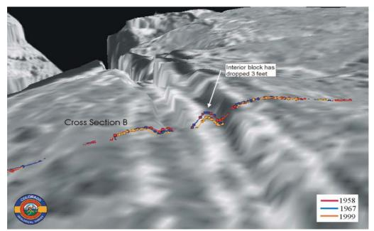
Figure 17. Main Graben Fissure above Upper Block. Photo drape is noticeably skewed by DEM conversion of poor quality photogrammetric contour lines at fissures that are more than 50 feet (15 m) deep along Cross Section B. Points of 1999 cross-section line (tan-colored) are a more accurate reflection of actual ground surfaces. Note 3-ft deflection downward of interior block of graben from 1967 to 1999, and little movement from 1958 to 1967. Also note left lateral movements of the Upper Block.
