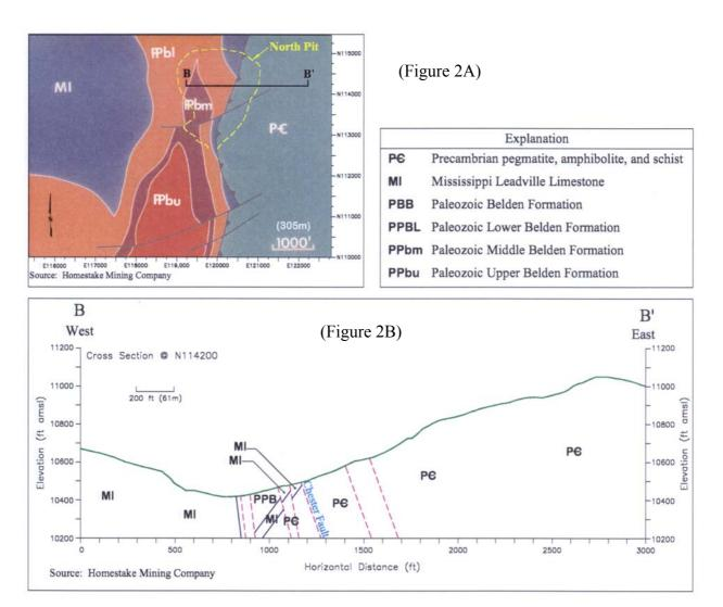
Figure 2. (A) Generalized geologic map of the North Pit area, and (B) generalized east–west, pre-mining geologic cross section through the North Pit area.
