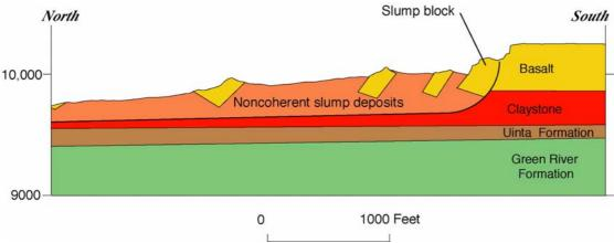
Figure 8. North-trending geologic cross section just west of Crater View, looking east (after Baum and Odum, 1996, section B-B').
