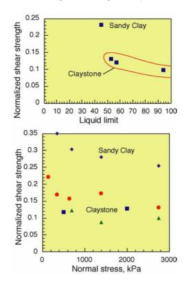
Figure 10. Relationships between normalized shear strength, liquid limit and normal stress of samples listed in Table 2. Normalized shear strength equals the shear strength divided by the normal stress.
