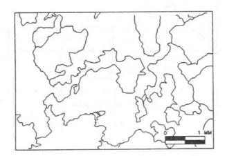
Figure 6. Tracing of Photomicrograph Mineral Boundaries, Pikes Peak Granite Tunnel Station 100+06.
