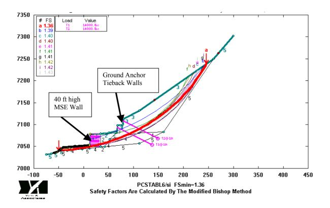
Figure 5. Generalized slope stability analysis depicting an MSE Wall with Ground Anchor Tiebacks for global stability.
