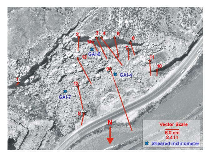
Figure 10. Movement vectors of prisms monitored from August 1999 through August 2002. Total movement vector for Prism #14 is smaller by comparison with the others on the cliff because it was installed 9 months later. The authors believe the Prism #10 vector is misleading. The vector is a mathematical calculation of initial and last-read measurements while the random range of multi-year measurements seems to show that the lower cliff is not moving).
