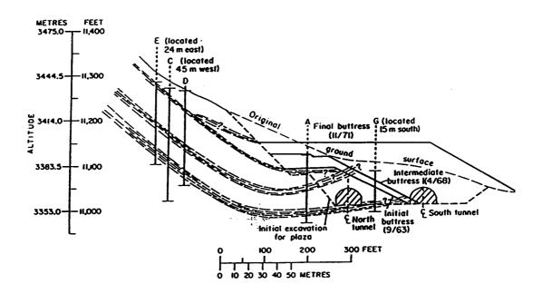
Figure 2. Generalized section through the toe of the landslide showing the approximate location of original ground surface, buttresses and major slip zones at eastern EJMT portal. (Fitzhugh, 1969).
