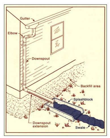
Figure 21. Components of a roof drainage system. From Noe and others (1997); modified from Jochim (1987).
