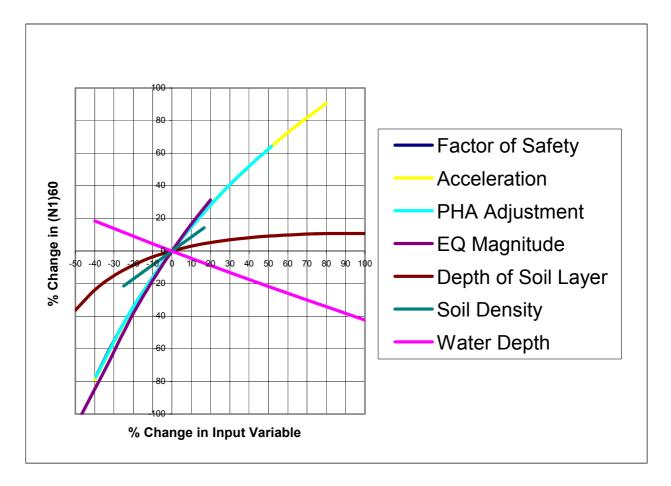
Figure 3. Sensitivity analysis of variables influencing liquefaction susceptibility. Input variables were modified and the effect was monitored on the critical  $(N_1)60$  value below which liquefaction would occur.
