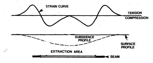
Figure 3. Subsidence and strain related to mining.
