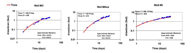
Figure 7. Theis curve fits for observation wells that exhibited a clearly correlated response to multi-well pump test, but for which only late time data were available.
