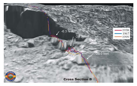
Figure 18. Cross Section B through the West Disturbed Block. White arrows and footage offsets are from elevation differences from 1958 to 1999 along the cross section line. Note blocks missing in center of image, which is reflected in the 1958 and 1967 plots. These large boulders have subsequently toppled into the Rubble Zone, and thus are not reflected in the 1999 plot data.
