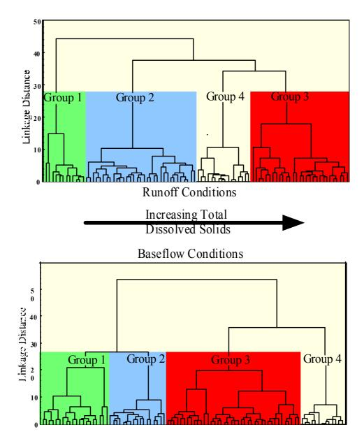
Figure 11a and b. Dendrograms of samples clustered using the HCA technique.
