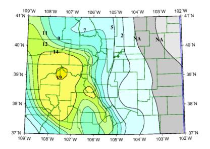
Figure 6. Liquefaction susceptibility related to earthquake accelerations generated by a  $\frac{2\%}{1000}$  Probability of Exceedance in 50 years event. Numbers shown on contours are critical (N<sub>1</sub>)60 values below which liquefaction of saturated, non-cohesive soils (<u>15% fines</u>) is expected. Base map is from USGS (2003).
