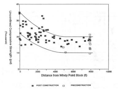
Figure 3. Pikes Peak Intact Compressive Strength versus Distance from the Windy Point Stock.
