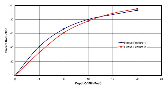
Figure 5. Reduction in predicted ground movement due to sub-excavation. Heave Feature 1 is 24 inches original height and Heave Feature 2 is 12 inches.
