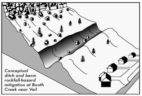
Figure 32. Berm and Bench as Rockfall Protection (Colorado Geological Survey, 1998).
