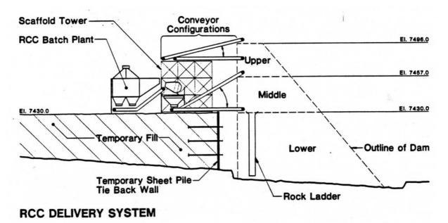
Figure 5. RCC Delivery System.
