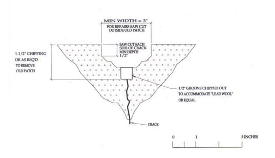
Figure 12. Schematic of Preparation of Concrete Lining at Crack
