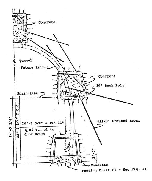
Figure 6. Zone II – Five Drifts and Rock Reinforcement Sta. 85+60 to 100+30.
