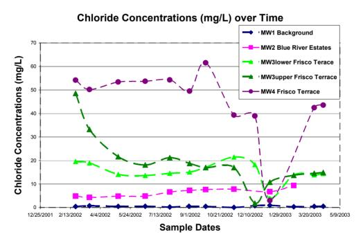
Figure 9. Chloride Concentrations mg/L in Ground water over Time
