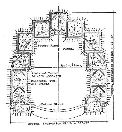
Figure 7. Zone II – Multiple Drifts Sta. 82+40 to 84+00.
