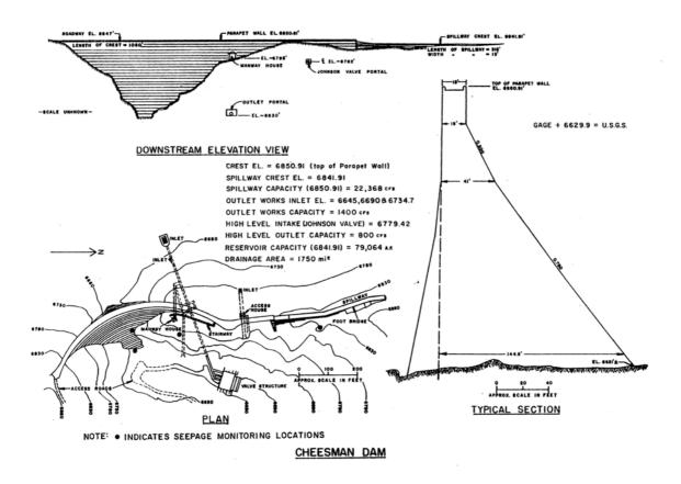
Figure 1. Plan, Profile, and Section of Cheesman Dam.
