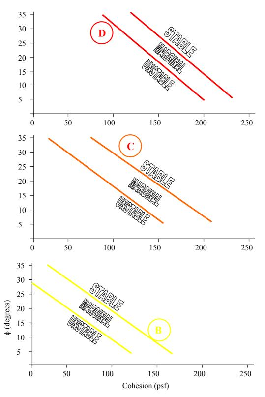
Figure 11. Soil strength influence on stability for small slopes (<100 cubic yds). To be used with Table 1. Conditions assigned to the letter "A" are expected to be stable.
