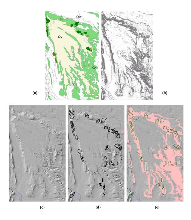
Figure 6. Mapping methodology demonstrated by GIS images of "The Mesa" area of Colorado Springs. Images shown are the geology and landslide deposits previously mapped by CGS (a), slope grade grid data (b), DEM based on 2-ft contours (c), finalized landslide inventory (d), and landslide-susceptibility map (susceptible areas shown in pink) (e).
