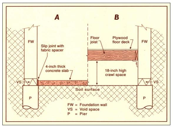
Figure 17. Two types of basement floor systems. (A) Floating slab floor. (B) Structural floor and crawl space. From Noe and others (1997).
