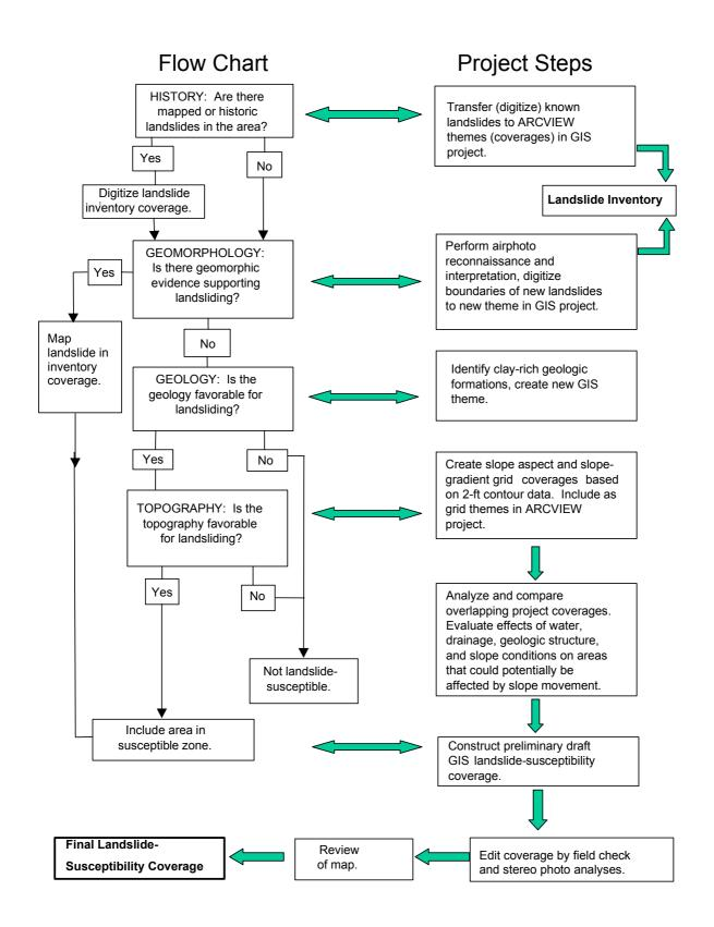
Figure 4. Flow chart showing decisions and related project steps for landslide-susceptibility mapping.
