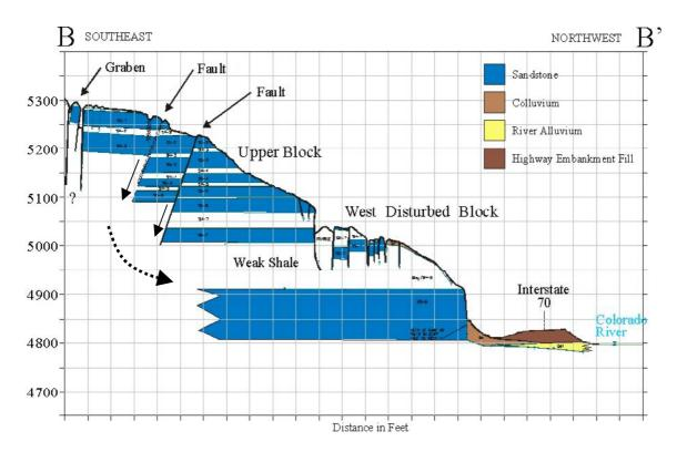
Figure 4. Cross section B. Cross-section line is shown on geologic map plate. Certain subsurface sandstone units are not shown in Upper Block. Note downdropped blocks of sandstone into underlying weak shale at West Disturbed Block and oversteepening of the shale slope that overlies the lower sandstone cliff at road level.
