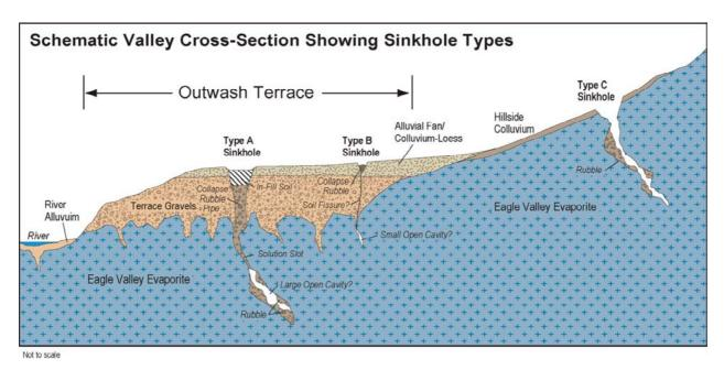
Figure 3. Schematic of sinkhole types (Modified from Mock, 2002).
