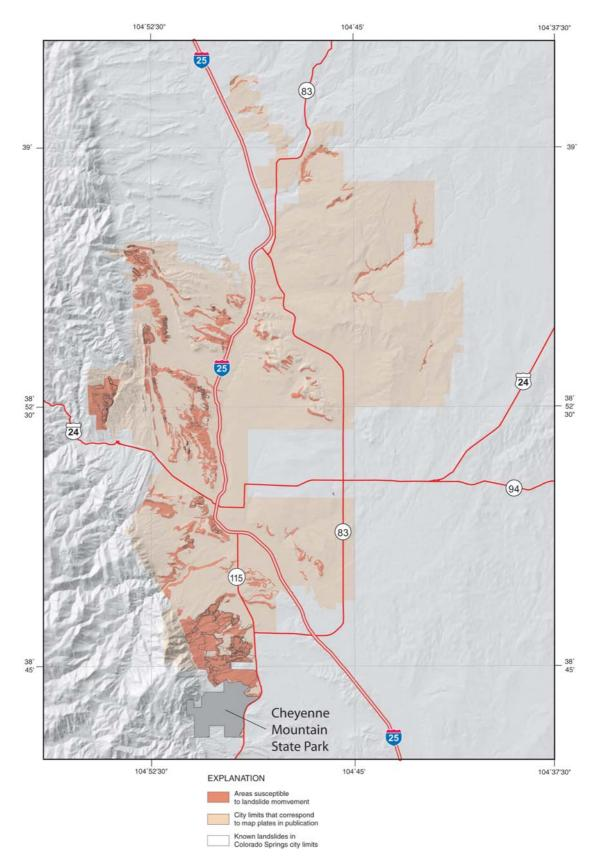
Figure 7. Colorado Springs landslide-susceptibility map.
