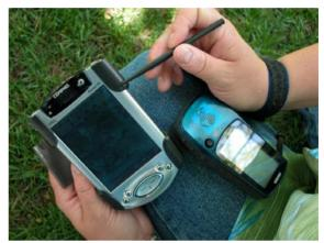
ArcPad handheld computer and GPS receiver in use. Arial photos can be loaded into ArcPad and used as a base map.
