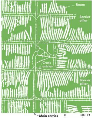
Figure 2. Possible layout of an early room and pillar mine, showing irregular room and pillar sizes.
