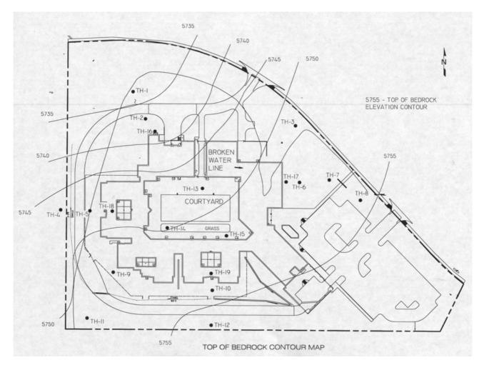
Figure 5. Commercial Structure No. 2 site plan with bedrock contours.
