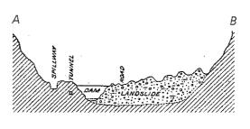
Figure 6. Original 1918 sketch map (a) and cross section (b) along line *A-B*, showing geologic conditions at Farmers Union (now Rio Grande) Dam on the headwaters of the Rio Grande River, southwestern Colorado (Atwood, 1918).
