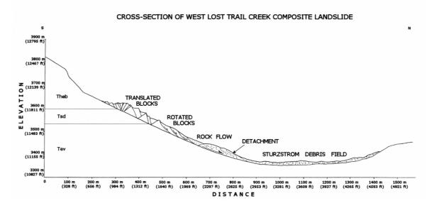
Figure 11. Cross section showing the 1991 landslide after movement ceased. The landslide deposits upslope of the sturzstrom debris field consist of a semi-coherent rock flow lobe, backrotated rock slump blocks, and a series of translated blocks.
