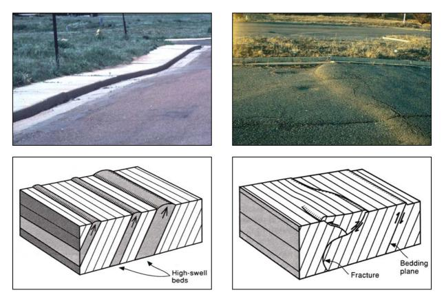
Figure 1. Examples and models of differential ground heaving caused by swelling of individual bedrock layers (left) and shear-slip movements along bedding planes or fractures (right). Block diagram models from Noe and Dodson (1999).
