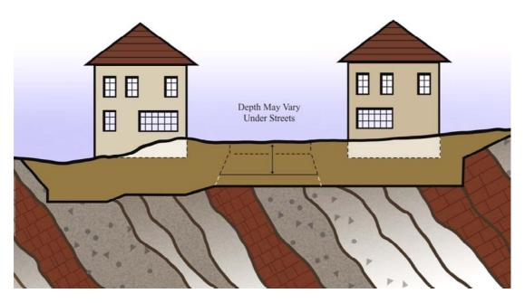
Figure 2. Typical deep sub-excavation profile. In Jefferson County, 10 ft of overburden soil or fill must separate foundations from the bedrock.
