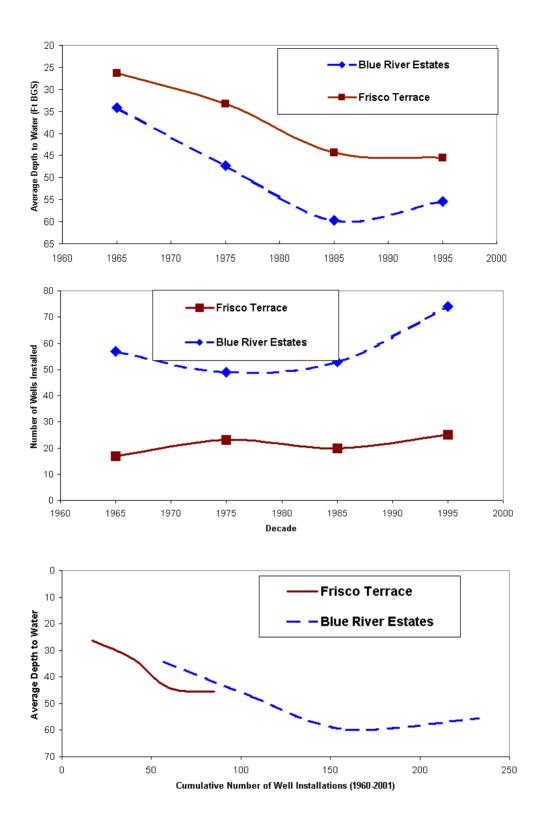
Figure 4. CSEO data for (a) Average water level by decade since 1960, (b) Number of wells installed by decade, (c) Cumulative number of wells installed vs. depth to water. BGS = below ground surface.
