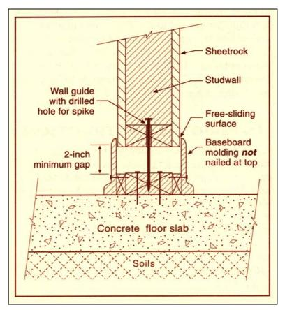
Figure 18. Detail of the bottom part of suspended, non-load-bearing interior wall. From Noe and others (1997); modified from Holtz and Hart (1978).
