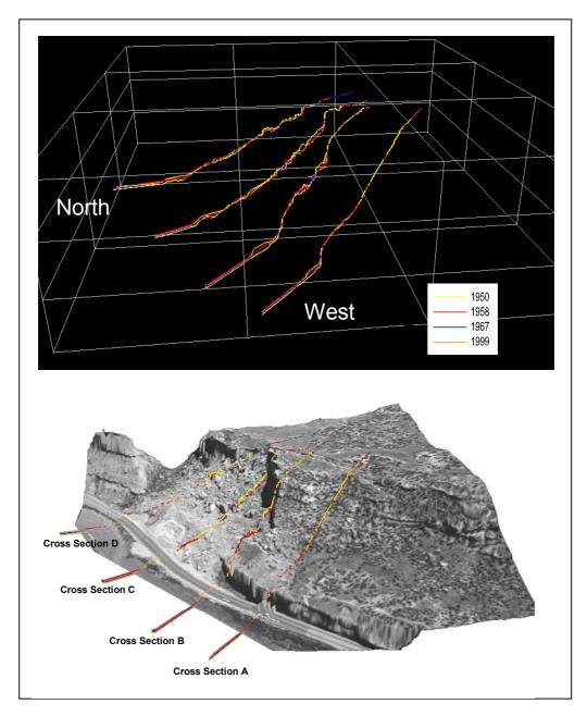
Figure 14. Projections of photogrammetric cross sections in 3D space and on DEM with draped 1999 aerial photograph. Cross sections B, C, and D correspond to same-lettered cross sections shown on geologic map. Cross section A is a control profile and does not correspond with profile A on the geologic map.
