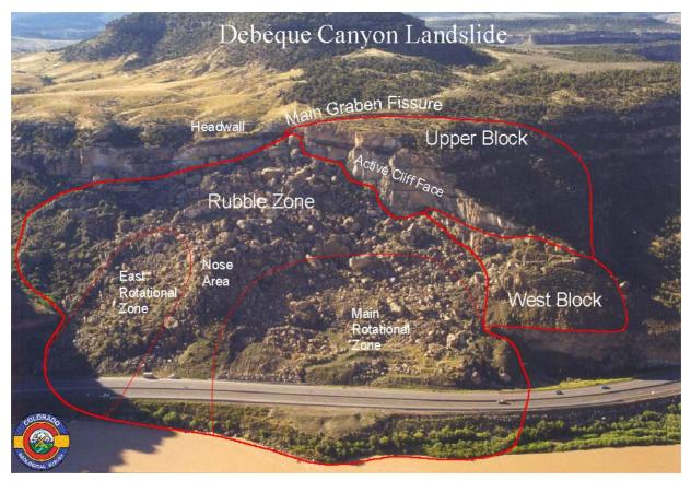
Figure 5. Oblique aerial photograph showing main morphologic divisions of landslide. Photo by J. White taken in 1999. View is to the south.
