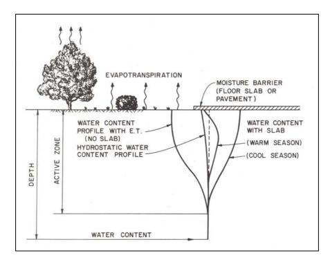
Figure 12. Soil profile showing the near-surface zone of moisture change, called the active zone. From Nelson and Miller (1992).
