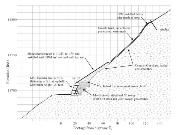
Figure 8. Schematic of slope-reconstruction design at the Big Cut.
