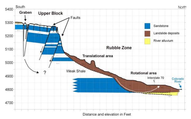
Figure 3. Cross section A. Cross-section line is shown on geologic map plate at end of paper. Certain subsurface sandstone units in Upper Block south of the faults are not shown.
