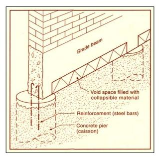
Figure. 15. Drilled pier foundation. From Noe and others (1997); modified from Holtz and Hart (1978).
