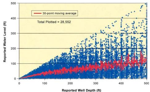
Figure 7. Scatter plot of reported water levels for specific well depths for wells completed in the Precambrian, crystalline-rock aquifer with a moving average trendline.
