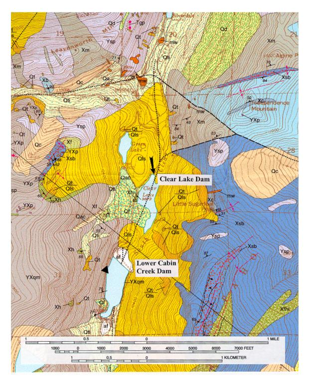
Figure 3. Surficial-geologic map showing location of Clear Lake Dam (arrow) on rock-slide deposits (Qls) and talus (Hammer (2002) along Clear Creek 2 mi (3 km) south of the town of Georgetown in the Colorado Front Range (after Widmann & Miersemann, 2001). Also shown is the location of Lower Cabin Creek Dam, the foundation of which reportedly was excavated through landslide deposits to bedrock
