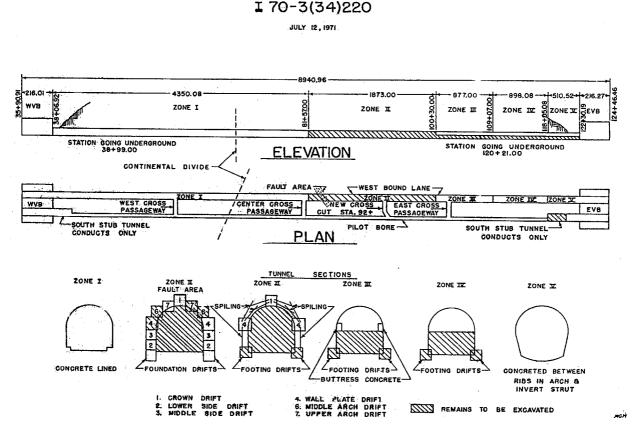
Figure 4. Elevation plans and profile for tunneling of the Straight Creek Tunnel.
