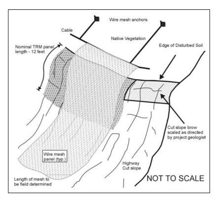
Figure 10. Schematic of cut slope brow treatment.
