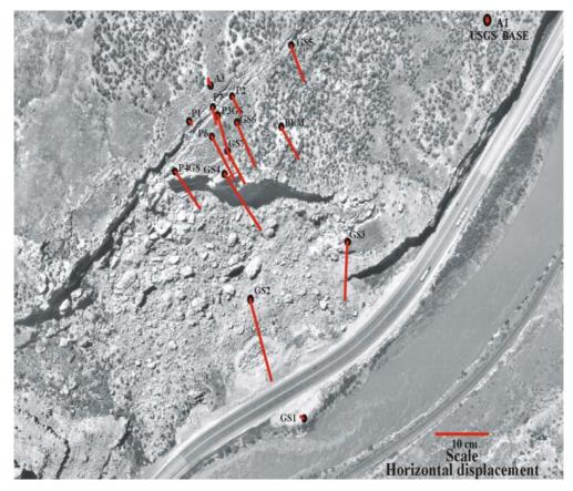
Figure 11. Movement vectors of GPS survey points measured from 1998 to 2002. Stations P1, A3, and GS1 vectors are within the error range (+/-1 cm) of the instrument.
