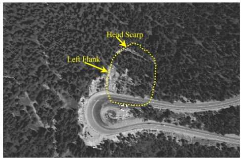
Figure 7. Landslide activated on July 4 weekend 1996. Pavement sheared and heaved as slide moved up to 6 ft (2 m) [CDOT, ca 1996].
