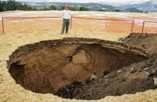
Figure 6. Photo on left is a void opened in river terrace gravels from utility excavation in the Roaring Fork Valley. Photo courtesy of Ralph Mock, Hepworth-Pawlak Geotechnical, used by permission. Photo on right is a sinkhole that opened in loess on a soccer field at Colorado Mountain College in February 2003. Maintenance staff has begun backfilling the crater.
