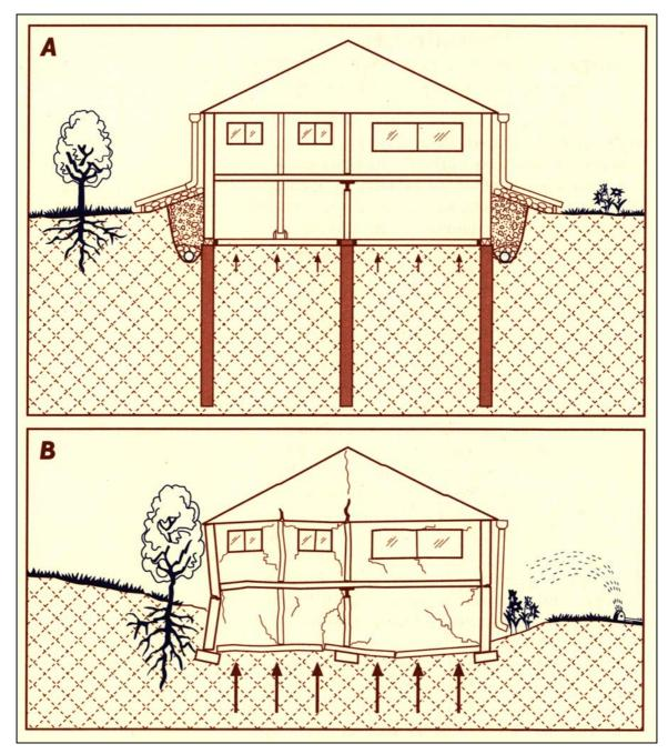
Figure 26. The results of (A) proper versus (B) improper design, construction, landscaping, and homeowner maintenance for homes built on expansive soil. From Noe and others (1997); modified from Holtz and Hart, (1978).
