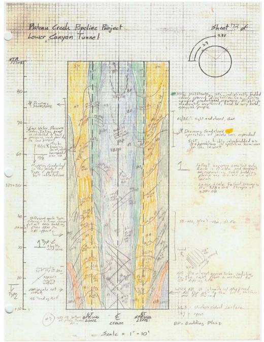
Figure 9. Example Tunnel Mapping Field Log.
