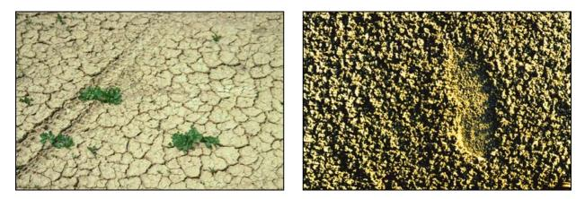
Figure 13. Evidence of expansive soils at the ground surface. (A) Small-scale desiccation cracks in soil containing expansive clay; note tire tracks for scale. (B) "Popcorn" texture in soil containing expansive clay having very high swell potential; note footprint for scale. From Noe and others (1997).
