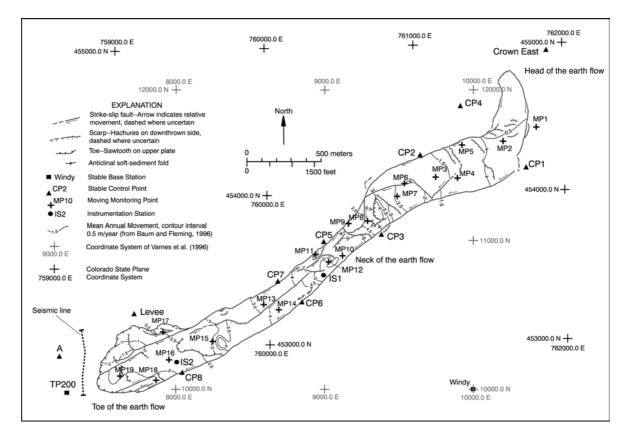
Figure 3. Map of the active part of the Slumgullion earth flow showing structural elements, contours of mean annual displacement, GPS base stations, control points, and monitoring points. Map modified from Baum & Fleming (1996).
