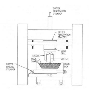
Figure 8. The Linear Cutting Machine (LCM).
