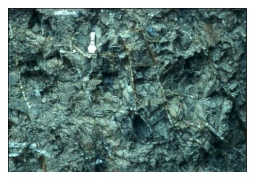
Figure 10. Highly fractured claystone of the Pierre Shale. These fractures contain veins of gypsum crystals, which are geochemical indicators of highly swelling bedrock. From Noe and Dodson (1999).
