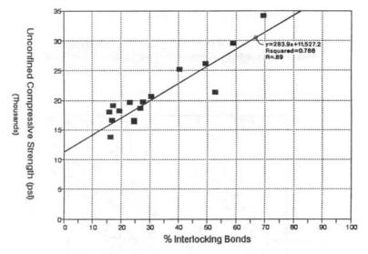
Figure 7. Pikes Peak Percent Interlocking Mineral Bonds versus Intact Unconfined Compressive Strength
