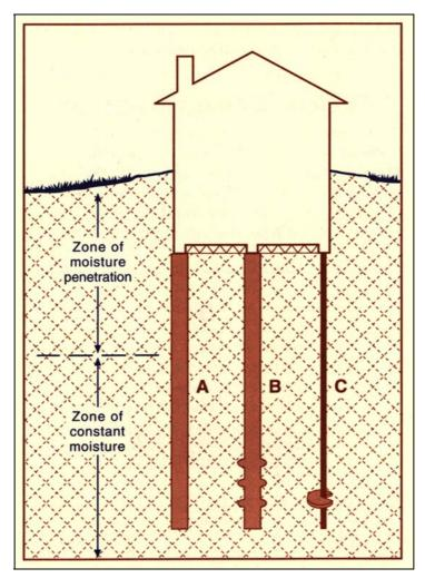
Figure 16. Three types of drilled piers commonly used in Colorado. (A) Straight-shafted concrete pier. (B) Concrete pier with grooves near base. (C) Helical steel pier. All piers should extend well below the anticipated zone of moisture penetration. From Noe and others (1997).
