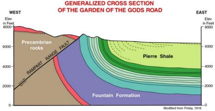
Figure 3. Generalized cross section through Colorado Springs showing bedrock dip along the Garden of the Gods road alignment (Himmelreich and Noe, 1999). Approximate location of section is shown on Figure 2.
