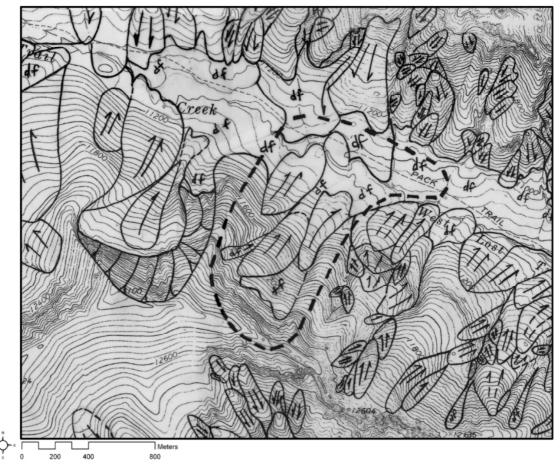
Figure 5. Landslide inventory map of the West Lost Trail Creek landslide area before the 1991 failure occurred. The heavy dashed line surrounds the 1991 landslide. Note the landslides which pre-existed the 1991 failure. The annotations "df" refer to debris fans and "tf" to talus fans", as introduced by Ives and Bovist (1978).
