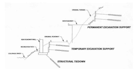
Figure 5. Anchor/wall configuration, from Kracum, (1993).
