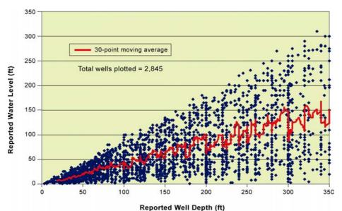
Figure 11. Scatter plot of reported water levels for specific well depths for wells completed in the Tertiary igneous rocks.
