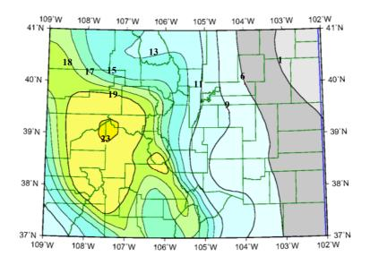
Figure 5. Liquefaction susceptibility related to earthquake accelerations generated by a  $\frac{2\%}{1000}$  Probability of Exceedance in 50 years event. Numbers shown on contours are critical (N<sub>1</sub>)60 values below which liquefaction of saturated, non-cohesive soils ( $\frac{5\%}{1000}$  fines or less) is expected. Base map is from USGS (2003).
