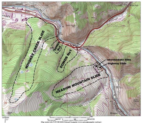
Figure 27. The Dowds Junction Landslide Complex (modified after Soule, 1988 Fig.1, and Jochim et al., 1988, Fig. 19).
