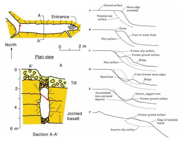
Figures 6 (Left) and 7 (Right). Figure 6. Sketch map and cross section of cavern at head of incipient slump block near Crater View. Figure 7. Schematic profiles of slump block evolution (after Baum and Odum, 1996).
