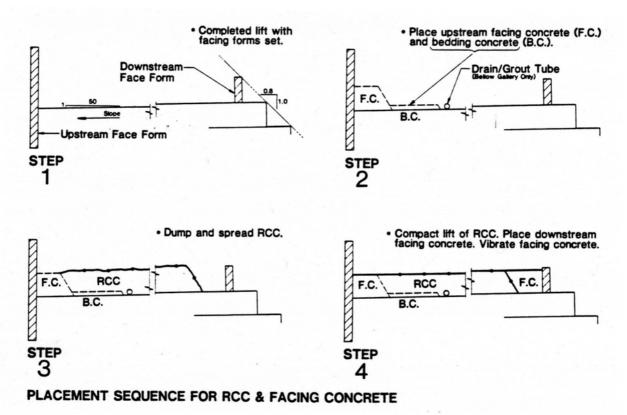
Figure 2. Placement Sequence for RCC and Facing Concrete.
