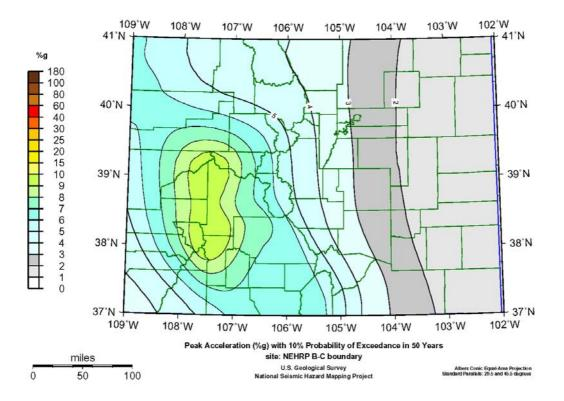
Figure 1. Expected earthquake accelerations with 10% Probability of Exceedance in 50 years (from USGS, 2003).
