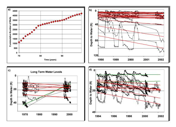
Figure 3. TCB wells and monitor-well water level trend lines (Red lines indicate decreasing water level, Green Lines indicate rising water level); a) number of wells in TCB; b) trend lines of monitor-well hydrographs in recent years (USGS, 2002; Hatch, 2002); c) trend lines of hydrographs in six wells with measurements over 30 years (USGS, 2002; Hatch, 2002); and d) trend lines of hydrographs in Parmalee Gulch from 1994 to 2002 (IHWD, 2002). Note scale changes between figures.
