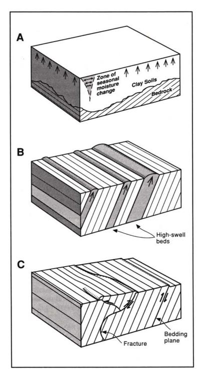
Figure 10. Different types of expansive soil and heaving bedrock. (A) General model for expansive soil, showing vertical heaving within the active zone of moisture change. (B) Symmetrical heave features caused by uneven swelling of bedrock layers. (C) Asymmetrical heave features caused by shear-slip movement along bedding planes or fracture surfaces. Image from Noe and Dodson (1999).
