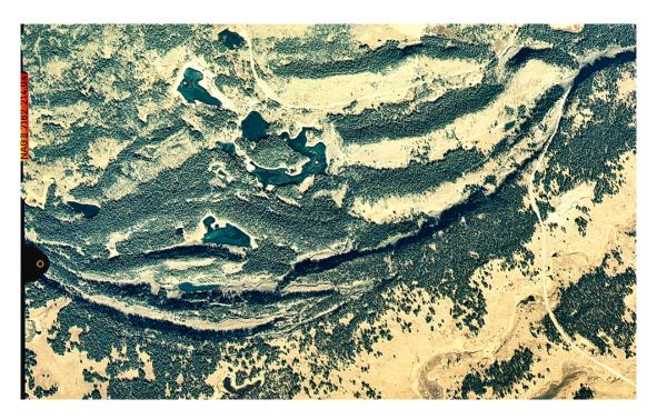
Figure 2. Aerial photograph showing distribution of slump blocks in the Mesa Lakes area, on the north side of Grand Mesa (USDA Forest Service Photograph 1388-6, 29 September 1988).
