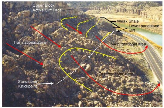
Figure 21. Oblique photo showing mechanism of landslide movements. Photo taken in 1999 by J. White. View is to the west.
