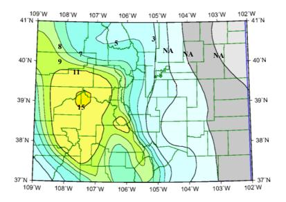
Figure 7. Liquefaction susceptibility related to earthquake accelerations generated by a  $\frac{2\%}{100}$  Probability of Exceedance in 50 years event. Numbers shown on contours are critical (N<sub>1</sub>)60 values below which liquefaction of saturated, non-cohesive soils (35% fines) is expected. Base map is from USGS (2003).
