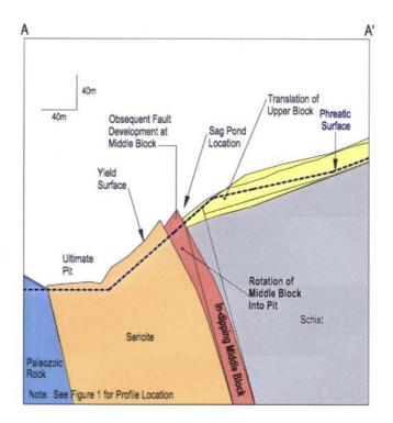
Figure 10. Post-displacement geotechnical model profile — deformation highly exaggerated.
