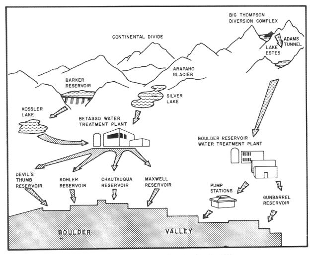
Figure 21. Boulder's water system (from City of Boulder, 1972).
