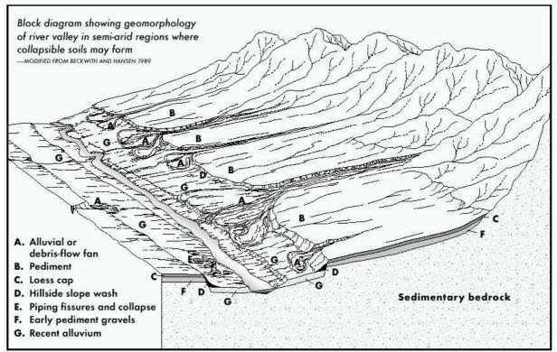
Figure 40. The geological setting producing hydrocompactible soils along Interstate 70 in western Colorado (Colorado Geological Survey, 2001; modified from Beckwith and Hansen, 1989).
