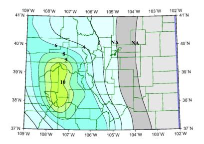
Figure 4. Liquefaction susceptibility related to earthquake accelerations generated by a  $\frac{10\%}{N_1}$  Probability of Exceedance in 50 years event. Numbers shown on contours are critical (N<sub>1</sub>)60 values below which liquefaction of saturated, non-cohesive soils (<u>5% fines or less</u>) is expected. Soils with 15 to 35% fines are not expected to liquefy under this size earthquake event. Base map is from USGS (2003).
