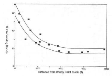
Figure 4. Pikes Peak Percent Interlocking Mineral Bonds versus Distance from the Windy Point Stock.
