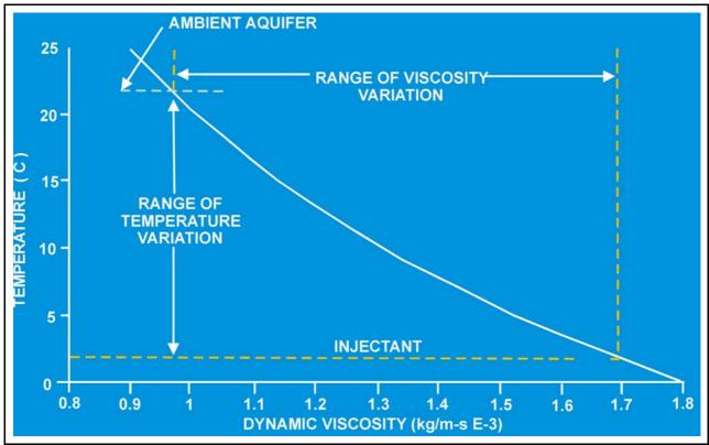
Figure 5. Effect of Temperature Change on Dynamic Viscosity
