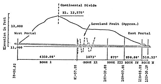
Figure 3. Generalized profile of the Straight Creek (Eisenhower) Tunnel (Leeds, 1974).
