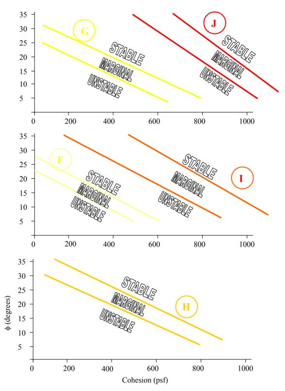
Figure 12. Soil strength influence on stability for large slopes (>10,000 cubic yds). To be used with Table 1. Conditions assigned to the letter "E" are expected to be stable.
