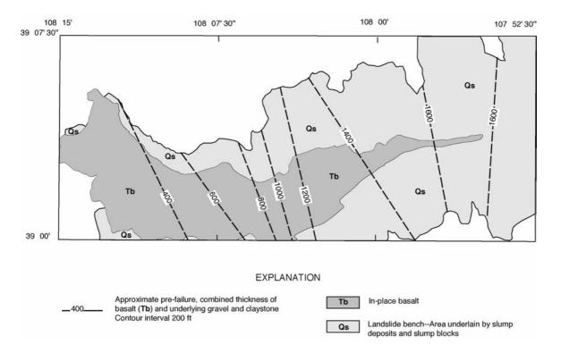
Figure 3. Approximate combined thickness of basalt and claystone involved in slumping. Area is that of Figure 1 (after Baum and Odum, 1996).
