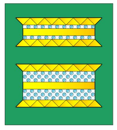
Figure 2. Expanding clay plates, as seen at a microscopic level. Circles indicate water molecules in the interlayer areas. Modified from Hart (1974).
