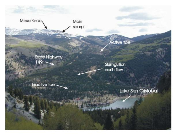
Figure 2. A view of the Slumgullion earth flow. View is to the northeast from southwest of the inactive toe and Lake San Cristobal.
