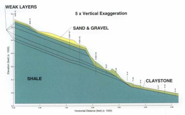
Figure 8. This cross section shown on Figure 6 has been exaggerated vertically so that the surficial deposits are visible; vertical lines indicate boring locations and depths, and the materials are generalized for clarity. The individual weak layers are shown thicker than the actual layers for visibility. This model does not include steeply dipping shale beds that may exist further west.
