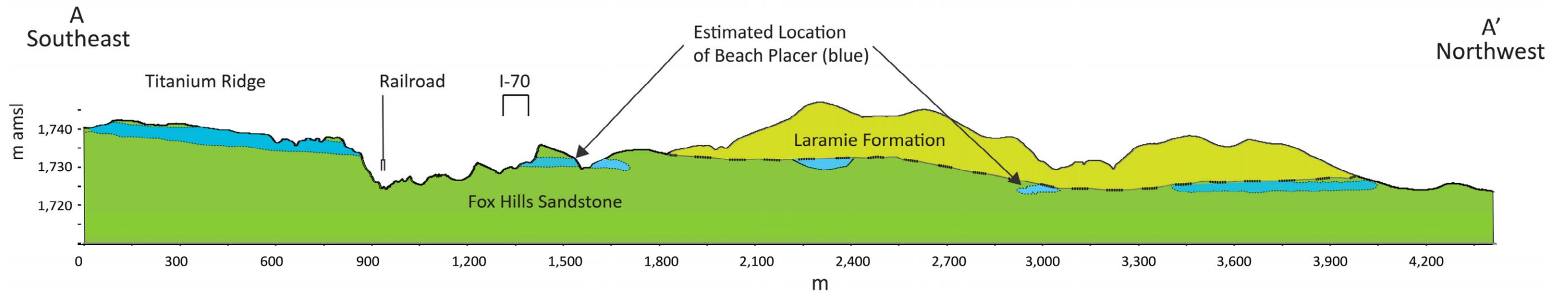
Figure – Generalized cross-section A-A' showing the location of Titanium Ridge to the southeast, Interstate 70 (I-70), and a beach placer trend along strike. Overlying surficial deposits not shown. Contacts and beach placers estimated from drilling information provided by others. m = meters, amsl = above mean sea level. The location of this cross section is shown on the “Cross Section Location Map” in this appendix.
