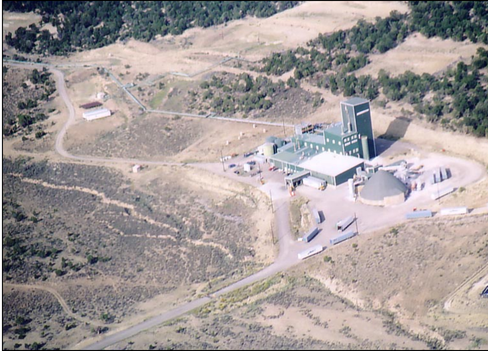
Figure 17. Aerial view of Natural Soda Inc's sodium bicarbonate plant in Rio Blanco County. Pipes that transport nahcolite-bearing solution from wells to the plant can be seen in the upper left. (Photo courtesy of Natural Soda, Inc.)
