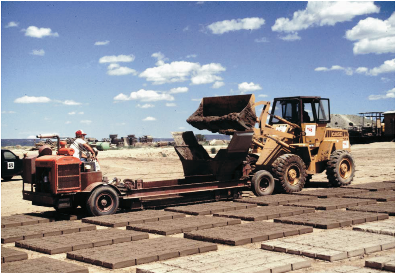
Figure 2. Front-end loader charging the hopper of an automatic adobe lay-down machine at the Adobe Factory, Alcalde, N.M. Once the hopper moves across the 25-space mold filling it, the lay-down machine picks up the mold and moves it to the next position leaving the adobes to dry.
