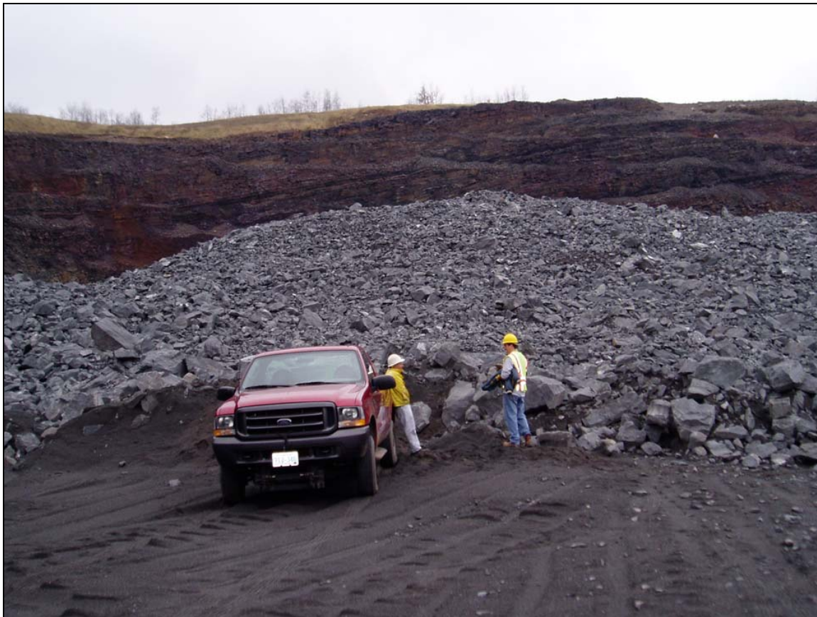
Figure 12. Sampling of post-blast taconite muckpile.
