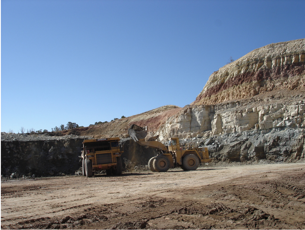
Figure 17. Phosphate mining at the Vernal mine of Simplot Phosphates LLC on the south flank of the Uinta Mountains in Uintah County, Utah. The quarry floor is formed by two feet of clay on top of the Pennsylvanian/Permian Weber Sandstone. Dark material is phosphorite ore and the lighter material overlying that is overburden.
