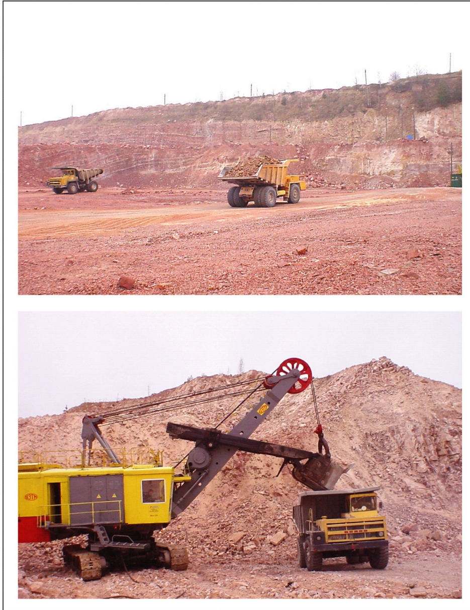
Figure 14. - Upper photo: Haul trucks in Ovruch quarry. Lower photo: Electric excavator loading quartzite into haul truck.
