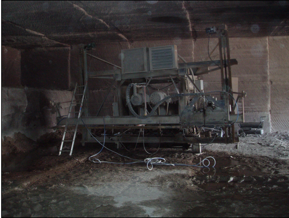
Figure 12. Water jet cutter at Colorado Rose Red Quarry, Larimer County.
