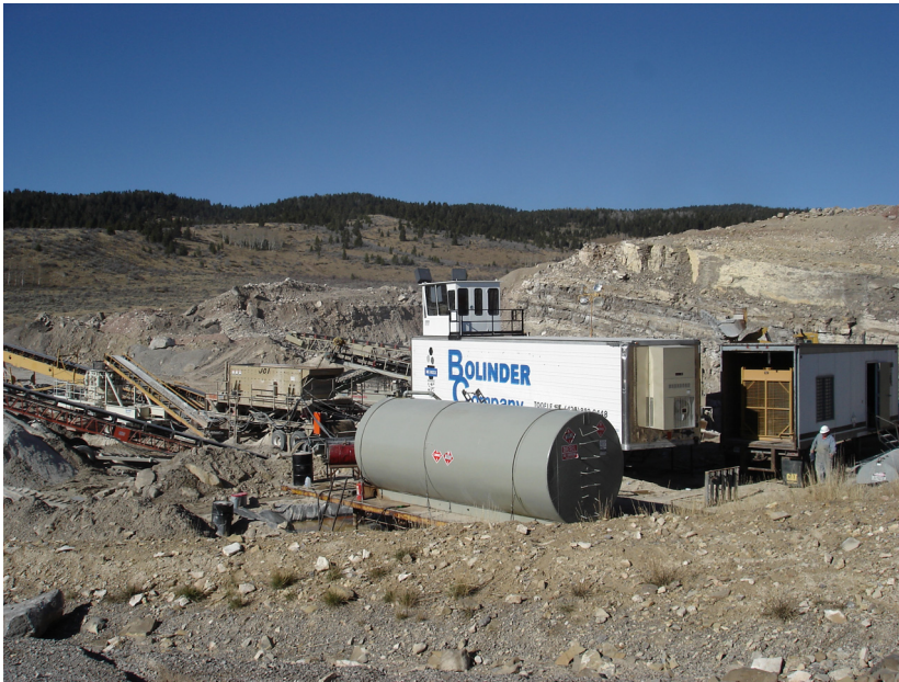
Figure 13. Mobil crusher processing Mississippian Madison Limestone at the Diamond Mountain limestone quarry on the south flank of the Uinta Mountains in Uintah County, Utah
