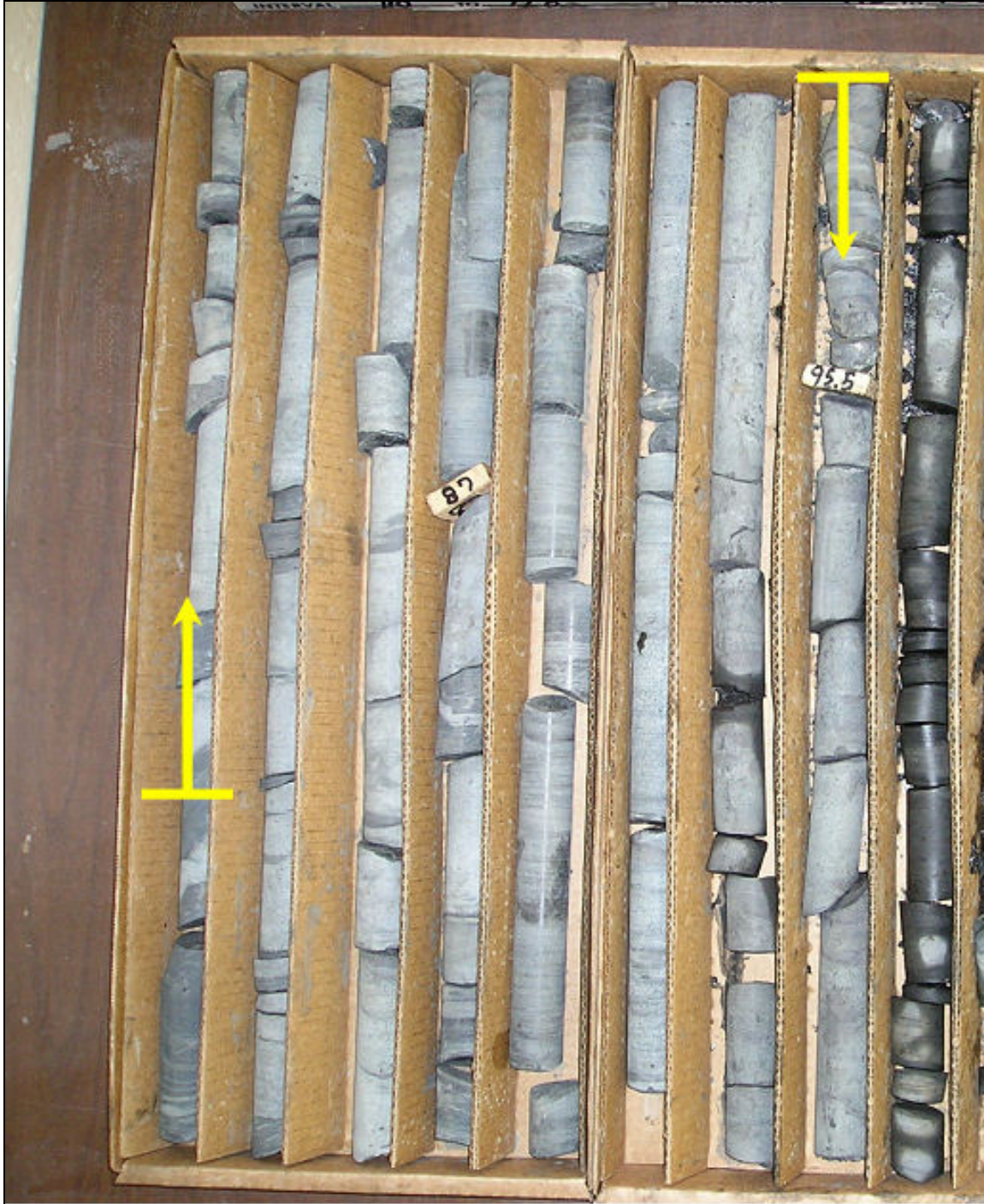
Figure 11. Drill core example of potential aggregate horizon between arrows. The interval represents channel deposition within the Lower Slaty submember of the Biwabik Iron Formation.
