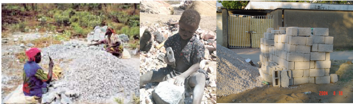
Figure 8. Aggregate produced by mainly women (a) and children (b) artisanal miners from the dolomitic marble in Lusaka for construction purposes (c).
