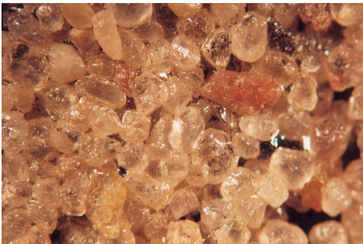
Figure 9. Immature sediment with angular fragments, mixture of sizes, various minerals, even mineral fragments.
