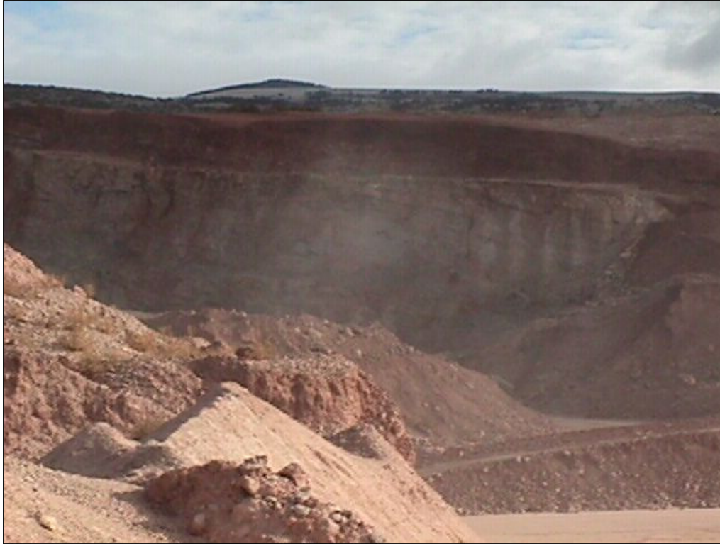
Figure 9. The failure to cleanly strip the overlying red Amsden Formation from underlying Madison Limestone results in Amsden material contaminating the Madison limestone product.
