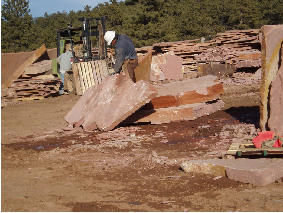
Figure 10. Hand trimming a piece of Lyons Sandstone at the Hotchkiss Sandstone Quarry, Larimer County.
