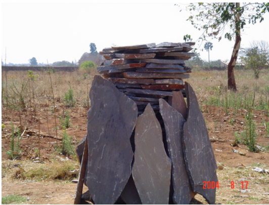
Figure 10. Flat stone exploited from Lusaka dolomitic marble for facing.
