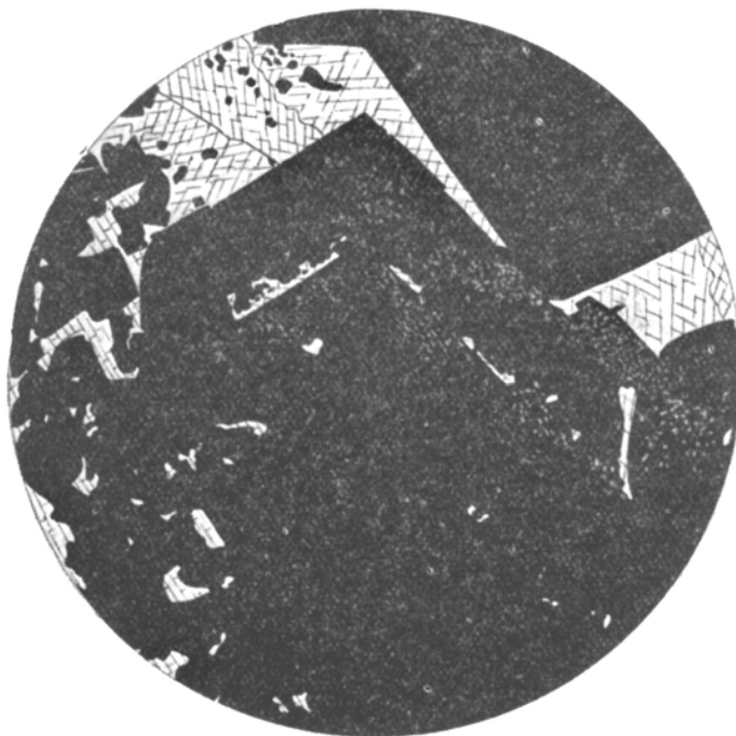
Figure 46. Thin section of magnetite with interstitial manganosiderite and zonal inclusions of the same mineral. Zonal aggregates of pyrite are also present. Magnified about 50 diameters.
