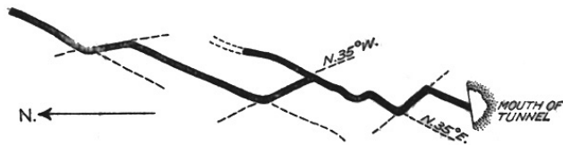
Figure 53. Vein with angular bends, common in many mining districts. (After J. D. Irving, U. S. Geol. Survey Bull. 478, p. 42, 1911)
