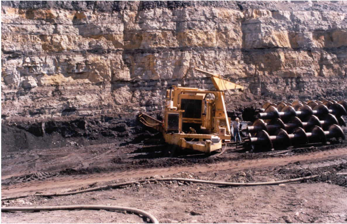
Figure 13. Auger mining methods in the Wadge coalbed, Yoast Mine. (Photograph courtesy of Seneca Mining Company)
