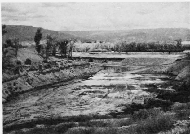
FIGURE 36. Whitewater Building Materials Corporation gravel pits west of Whitewater. This eastward view shows various stages of operation: revegetated fill in foreground; in near center, excavated pit undergoing backfill (at right), gravel and overburden thickness visible at left; at top center are excavation machinery and stockpile in the active pit. Overburden has been removed in back of machinery in preparation for mining.
