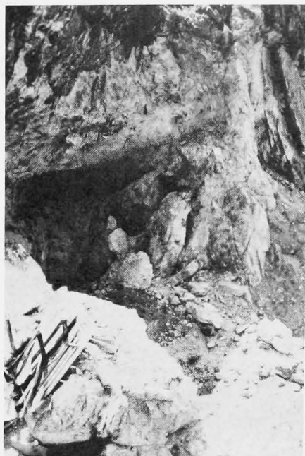
FIGURE 27a. Main cut at the Que #2 pegmatite mine in Ladder Canyon southwest of Grand Junction. Although the mine originally produced muscovite, only decorative quartz has been mined in recent years. This view eastward into the cut is approximately normal to the trend of the zoned pegmatite.
