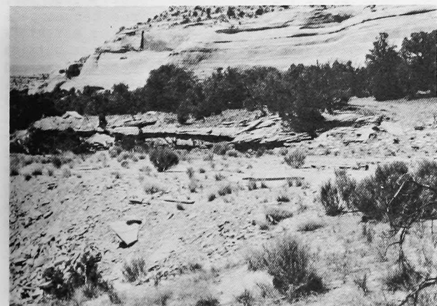
FIGURE 30. Sandstone quarry near Long Mesa. Flagstone here was quarried from a low bench in the Kayenta Formation. In contrast to the evenly bedded flagstone, note the strongly cross-bedded sandstone immediately above the quarry face. Scrap rock lines the stream bank in the foreground. The massive Entrada Sandstone forms the prominent smooth ledge in the background.
