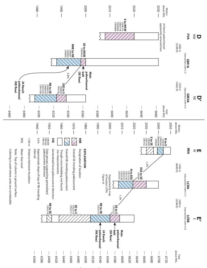
FIGURES 17&18. CROSS SECTIONS D-D' AND E-E' SHOWING CASTLEWOOD CANYON REACH OF MAIN PALEOCHANNEL AND ALSO JA RANCH PALEOCHANNEL.
