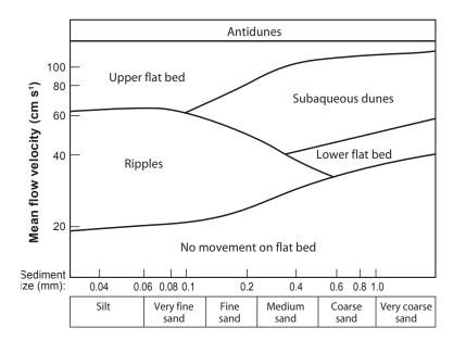
FIGURE 3. BEDFORM STABILITY DIAGRAM (FROM NICHOLS, 2009). (Used with permission of John Wiley & Sons Ltd.)
