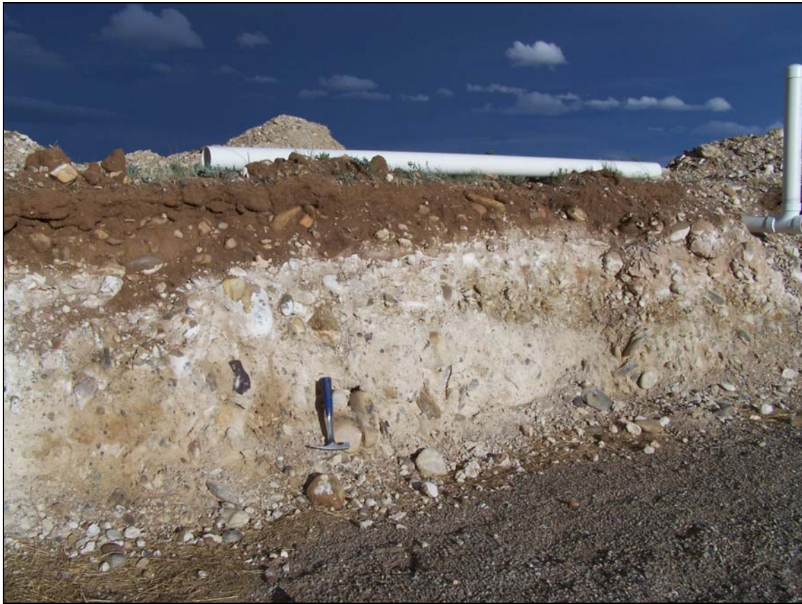
Figure 8. Stage III to weak stage IV carbonate horizons are typical of alluvial unit four. Photograph shows exposure of unit Qa4y in excavation for leach field of septic system located at approximately UTM coordinates 421920 m E, 4325510 m N. White pipe rests on ground surface.
