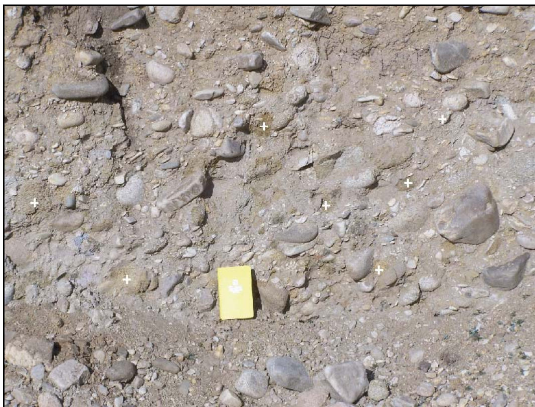
Figure 10. Weakly lithified, silty, sandy, cobble and pebble conglomerate in the Wagontongue Formation exposed in a small excavation at about UTM coordinates 422070 m E, 4321970 m N. View is to east-northeast, parallel to the direction that the beds dip. Small white “plus signs” denote several of the many decomposed clasts in the unit. Note the shingling or imbrication of clasts, which suggest the gravel was deposited by a stream flowing from left to right. Yellow notebook is 5 x 7.5 inches.
