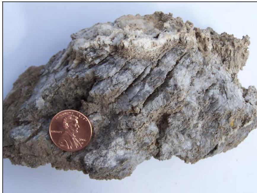
Figure 21. Gypsum in the evaporite facies of the Minturn Formation locally is partially dissolved along laminations. Dissolved gypsum is commonly re-precipitated in voids, as seen on the top of this specimen. Gypsum-rich precipitate also overlies outcrops of some gypsum beds, for example on the south and west sides of Bare Hill.
