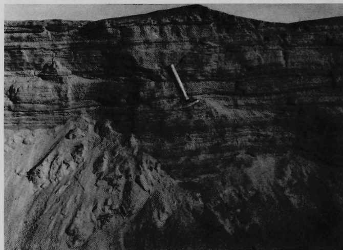
Figure 5. Fountain Sand and Gravel Company hydraulic fracturing sands in El Paso County. This deposit supplies the petroleum industry in the United States and Canada with coarse-grained quartz sands that are used to increase the recovery of oil. The pit is located 1 mile east of the south entrance of the U. S. Air Force Academy. Photograph by P. C. Wicklein.
