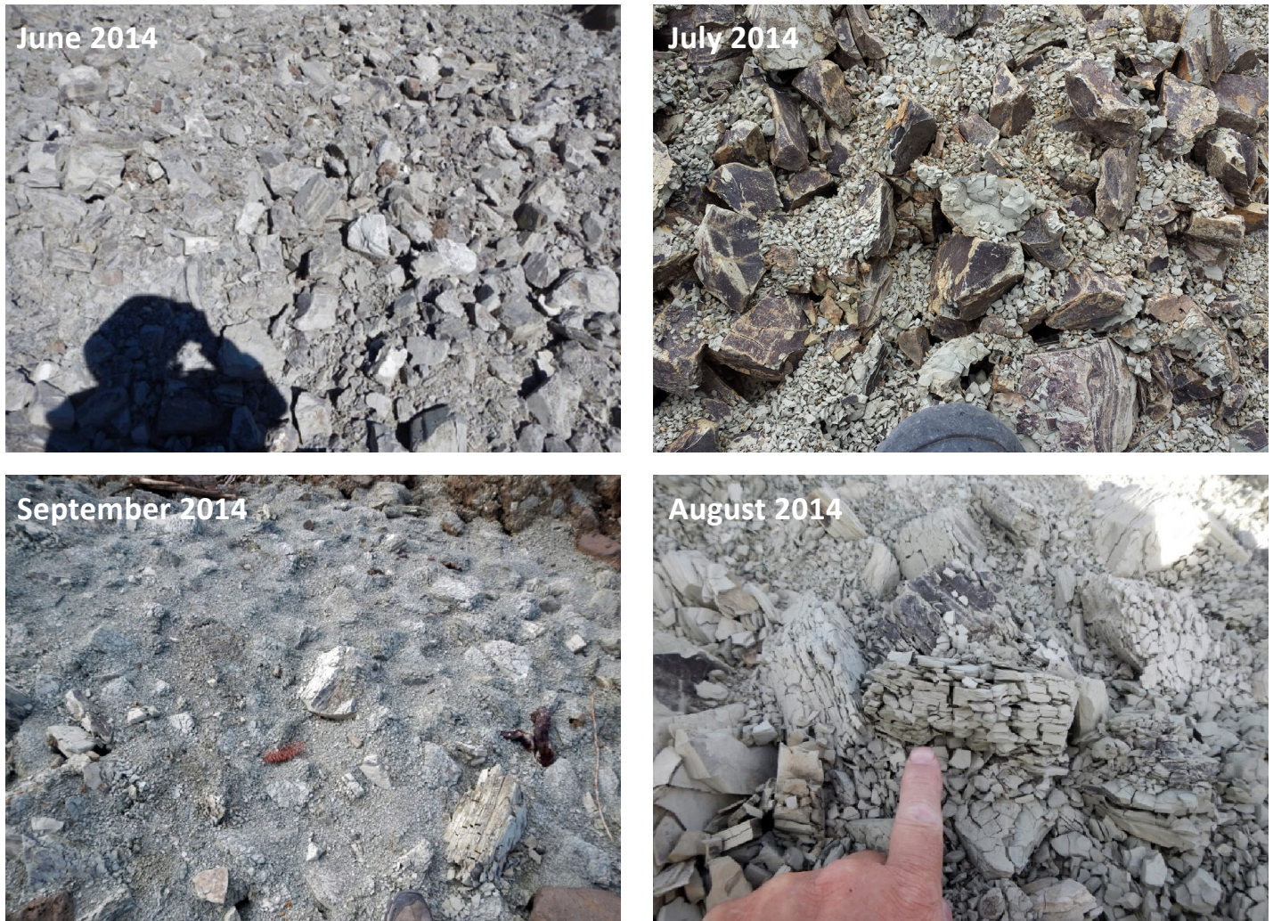
Figure 16. Rapid slaking of Green River Formation claystone and marlstone clasts in the WSCL debris field. Note surface staining of clasts and progression, clockwise from upper left, of rock disintegration in less than 4 months.
