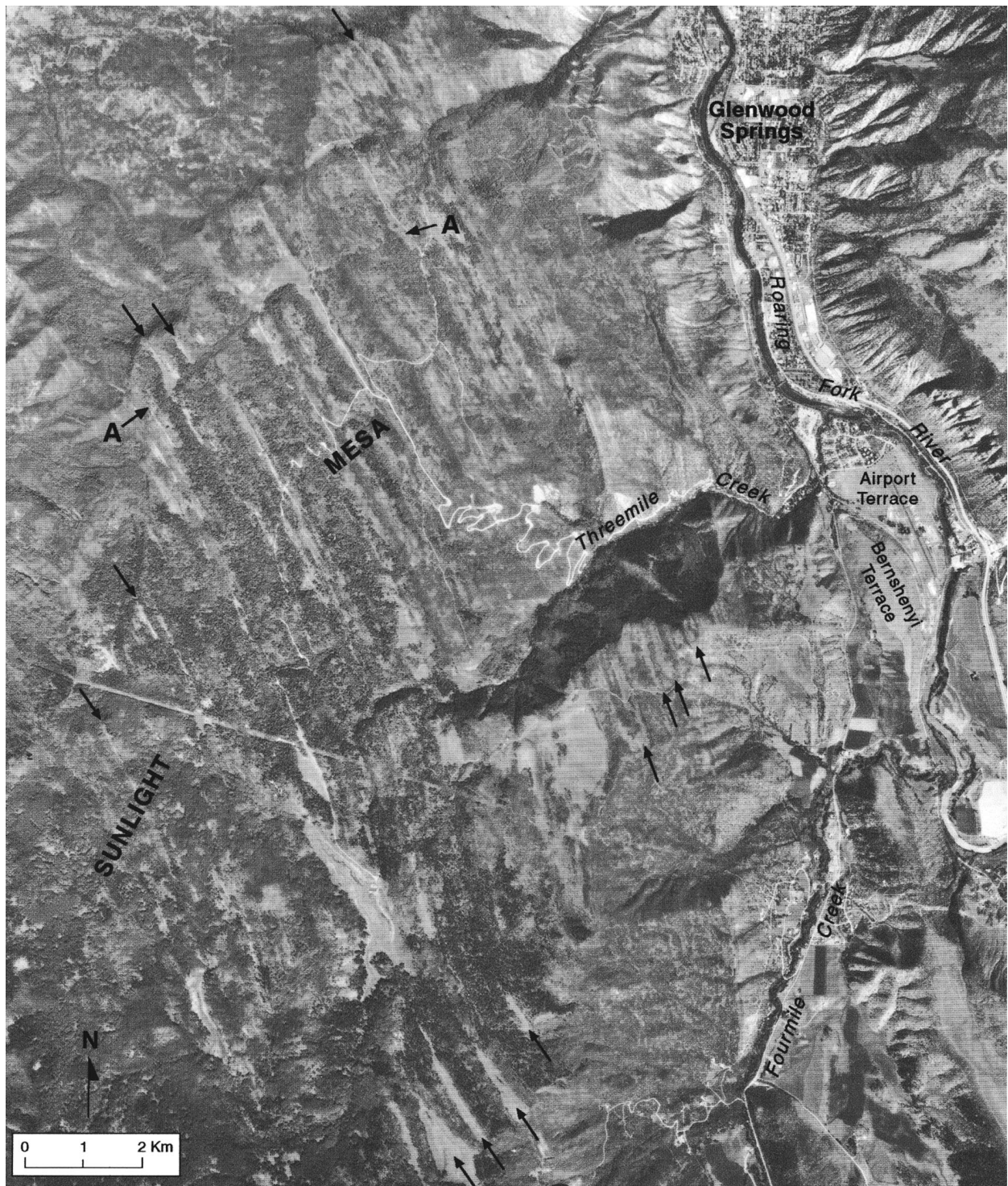
Figure 5. Vertical aerial photograph of the Sunlight Mesa area (National Aerial Photography Program [NAPP] photo 6716-41), where flexural-slip faults cut Miocene volcanic rocks that overlie an angular unconformity eroded across west-dipping sedimentary rocks in the Grand Hogback monocline. Note the prominent, parallel, northwest-striking, light-colored lineaments that are linear grassy valleys (some are marked by arrows). Each valley is underlain by a west-dipping normal fault related to relaxation of the monocline. The linear dark areas between the valleys are ridges formed by fault blocks capped by east-dipping volcanic rocks. Arrows labeled "A" indicate ends of a cross fault that cuts upper Quaternary deposits. Bershenyi terrace has been folded by Pleistocene diapirism. Town of Glenwood Springs in upper right. Scale and north arrow are approximate.
