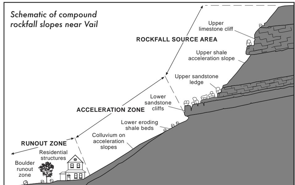
occurred there. Since then, the town and property owners in Vail Village filing 12 formed a Geologic Hazard Abatement District (GHAD). The district has mitigated much of the hazard by constructing a ditch and berm on the slope above the residential area. The ditch and berm configuration has been very effective for rocks that continually fall from the cliffs of the Minturn Formation (see below).
