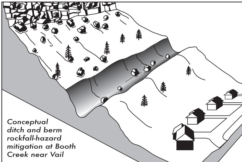
*Conceptual ditch and berm rockfall-hazard mitigation at Booth Creek near Vail*
